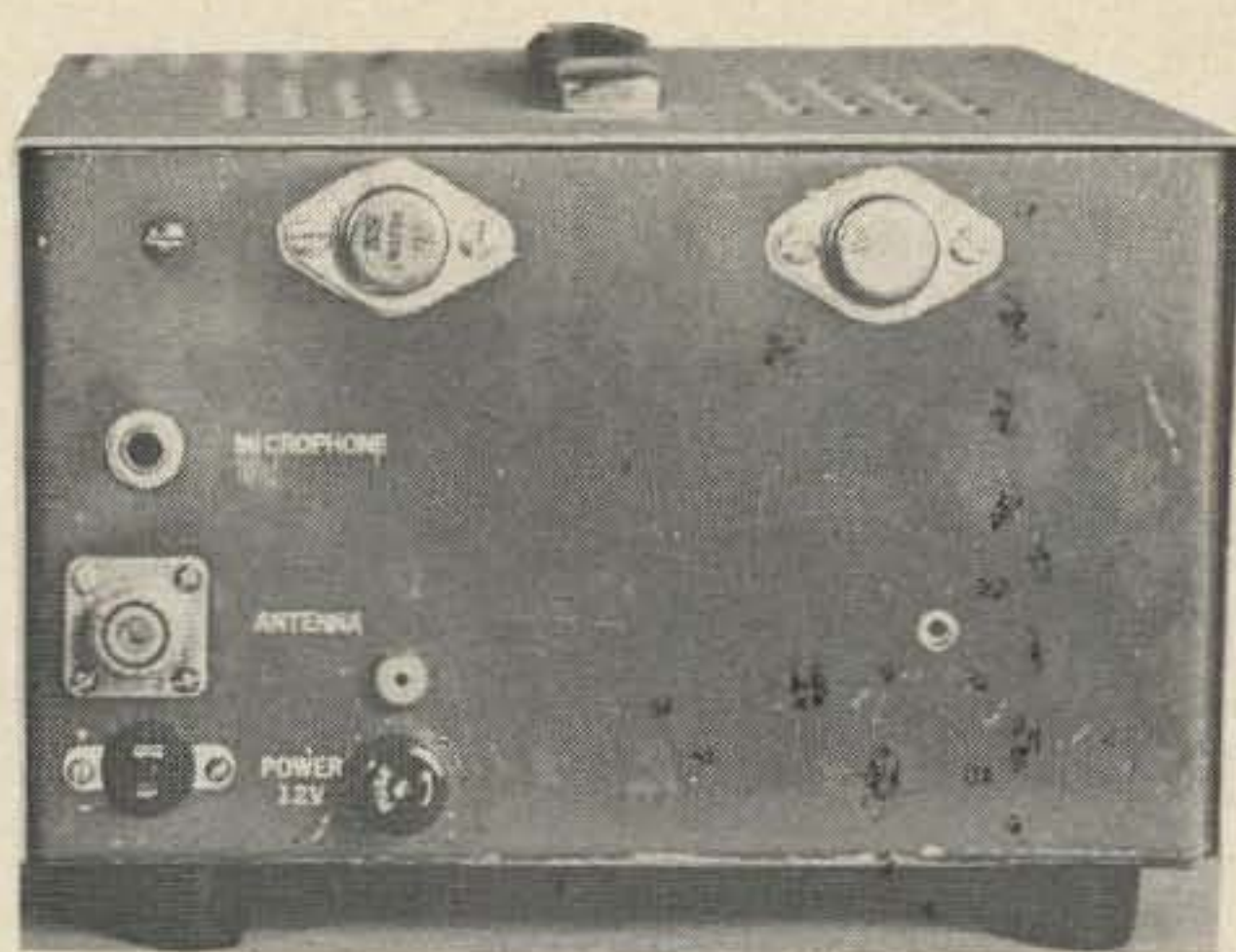
Rear view showing the connectors for power, antenna and microphone. The two LM309 regulators were mounted after scraping away enough paint to get good thermal contact with the chassis.
