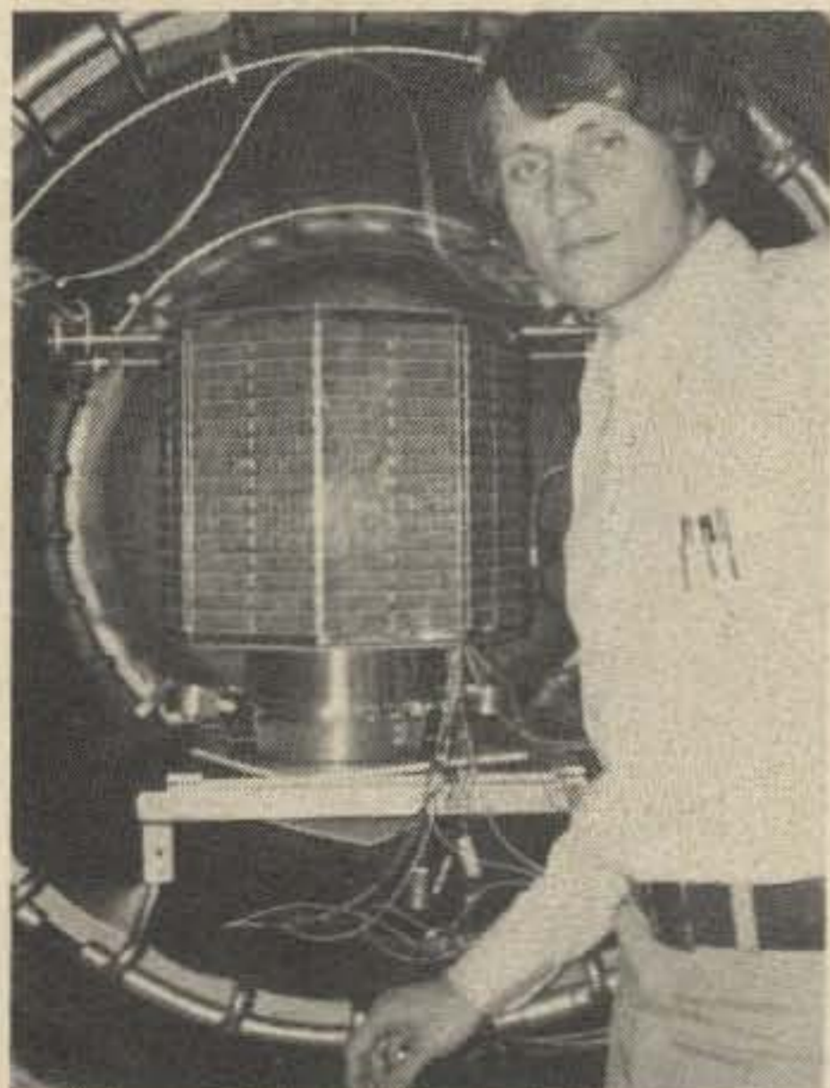
Jan King W3GEY, A-O-B Project Manager installing A-O-B in Thermal Vacuum for testing.
