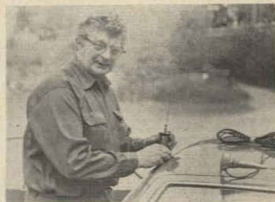
Gam Antenna Installed — Andy Nuttle of Gam in Manchester NH is installing one of his new two meter antennas on the 73 Test Car — the Datsun 240Z. Andy makes just about every part of these antennas himself in his highly automated factory. The SS-2 is designed to have a particularly low angle of radiation, thus squirting the rf in the desired direction and not up toward some passing plane as with some of the 2m antennas in use today.
