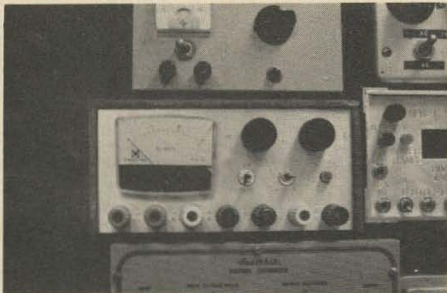
The Universal Power Supply. It has 3 fixed voltages and 2 regulated. See text for details.
