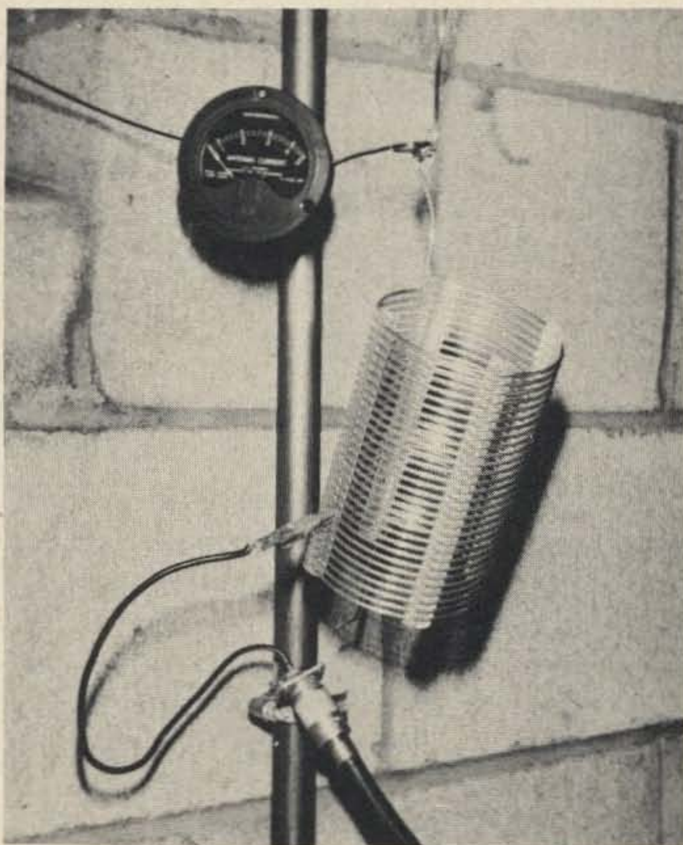
The coil at the feedline end is not grounded but the coax connector can be easily strapped right to a nearby pipe.
