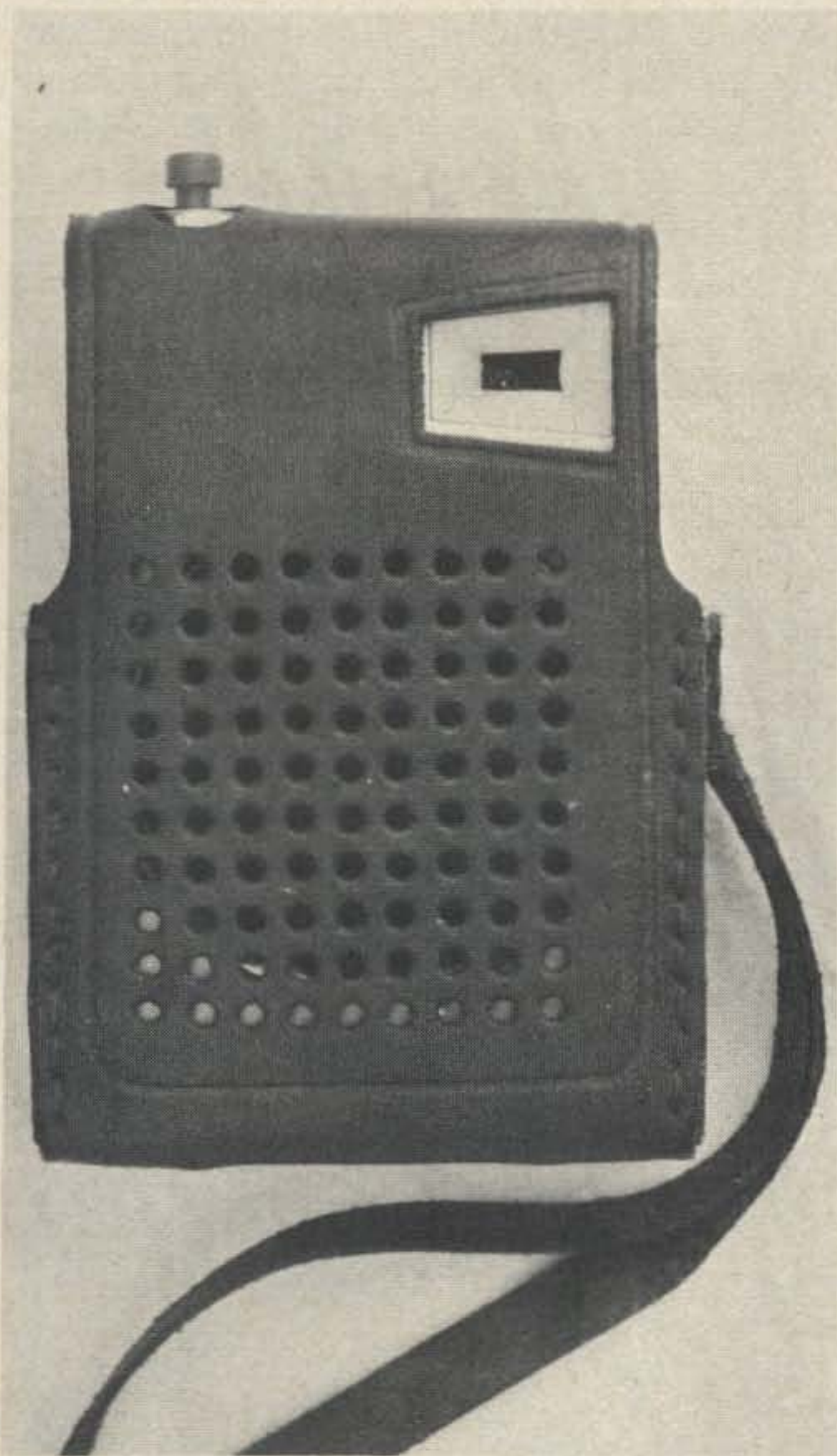
A phase locked loop tone oscillator built in an old 6 transistor radio. The only external difference is the lack of a tuning capacitor and an added pushbutton.
