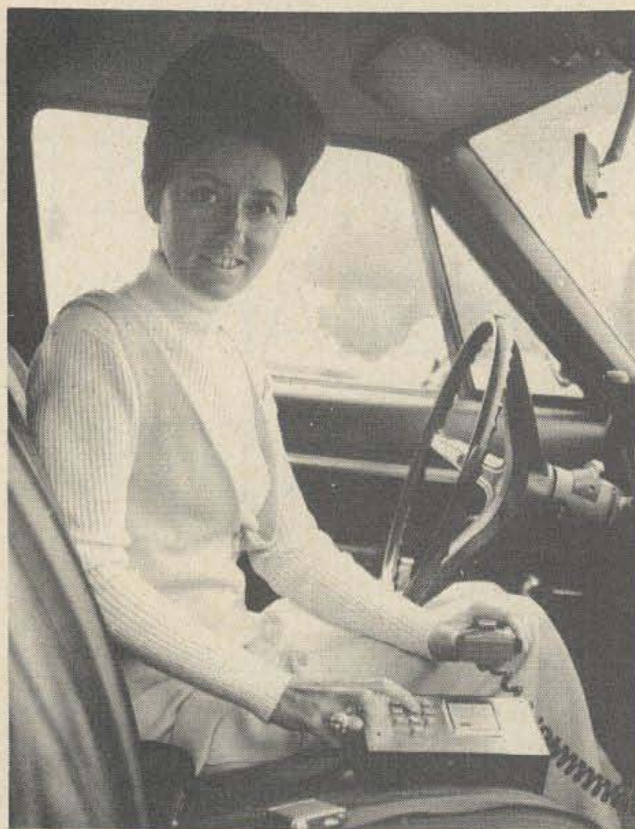
A touch tone can also be used with a borrowed radio audio section. This unit does double duty with both a touch tone and PLL oscillator feeding through the same audio unit. Pushing the buttons is the author's wife, WA7NDK.
