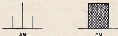
Fig. 2. Spectrum distribution charts for AM and FM show that AM occupies fixed positions in the rf spectrum, while an FM signal appears to vary in frequency over a band of closely related frequencies. With most receivers, the AM spectrum distribution would appear to be a single point rather than the three points shown.
