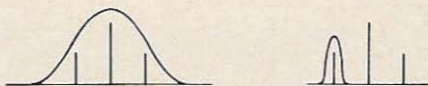
Fig. 3. AM appears to be a single-frequency signal to almost all receivers, and many spectrum analyzers, because the receiver's selectivity curve is so broad as to include the carrier and all sidebands as shown at left above. An extremely selective receiver (right), or analyzer, is capable of selecting any one component of the complete signal and isolating it.
