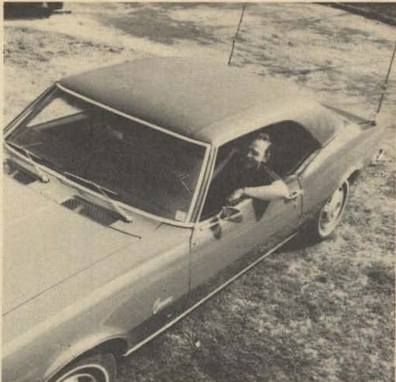
Twin antennas mounted on the rear cowl keep the author's installation from looking junky. Inside the car, the only visible evidence of a rig is the "Princess" telephone, mounted to the console and modified to serve as a "control head."
