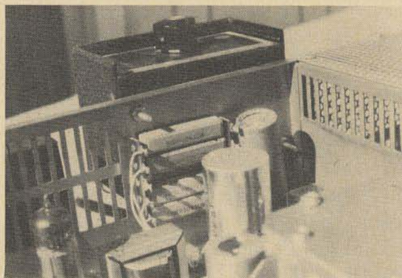
Inside view of 250-C showing the two bolts to mount the noise silencer (the other one is just right of the electrolytic).
