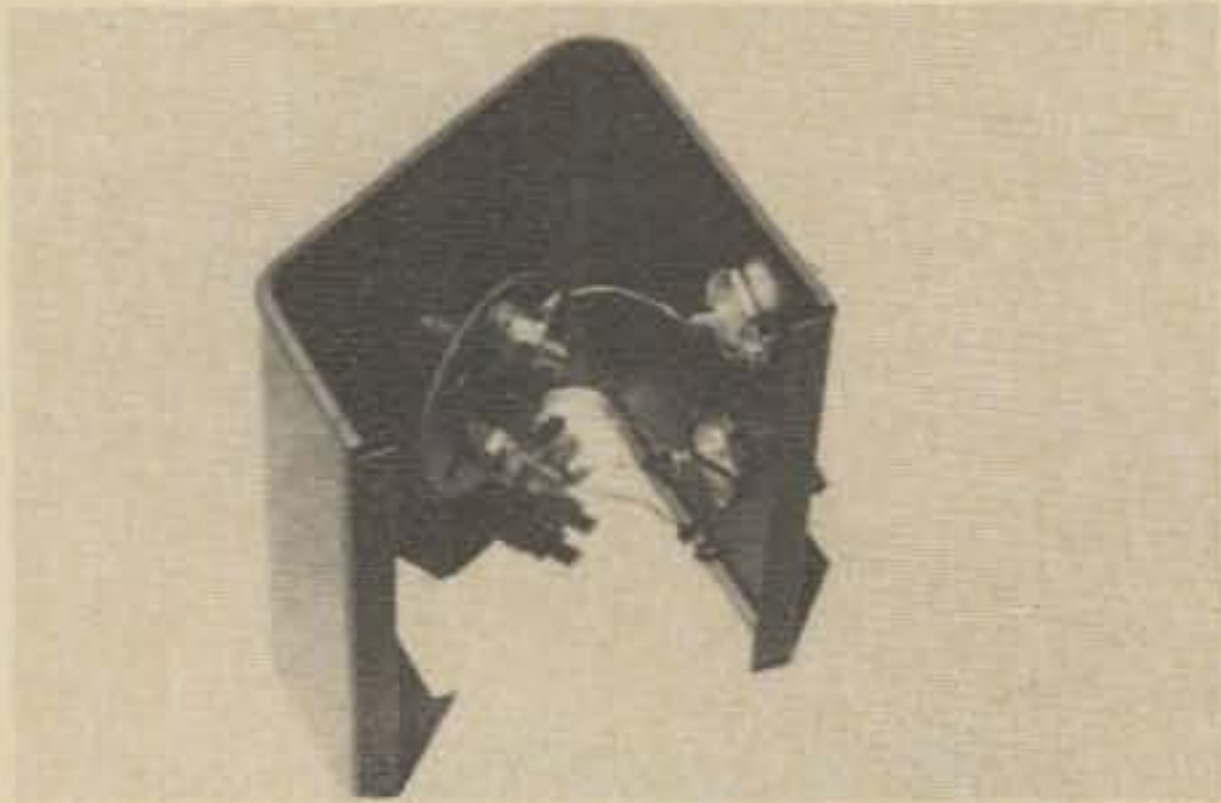
Inside wiring is extremely simple. Note ground wire installed to insure continuity of the shield circuit.
