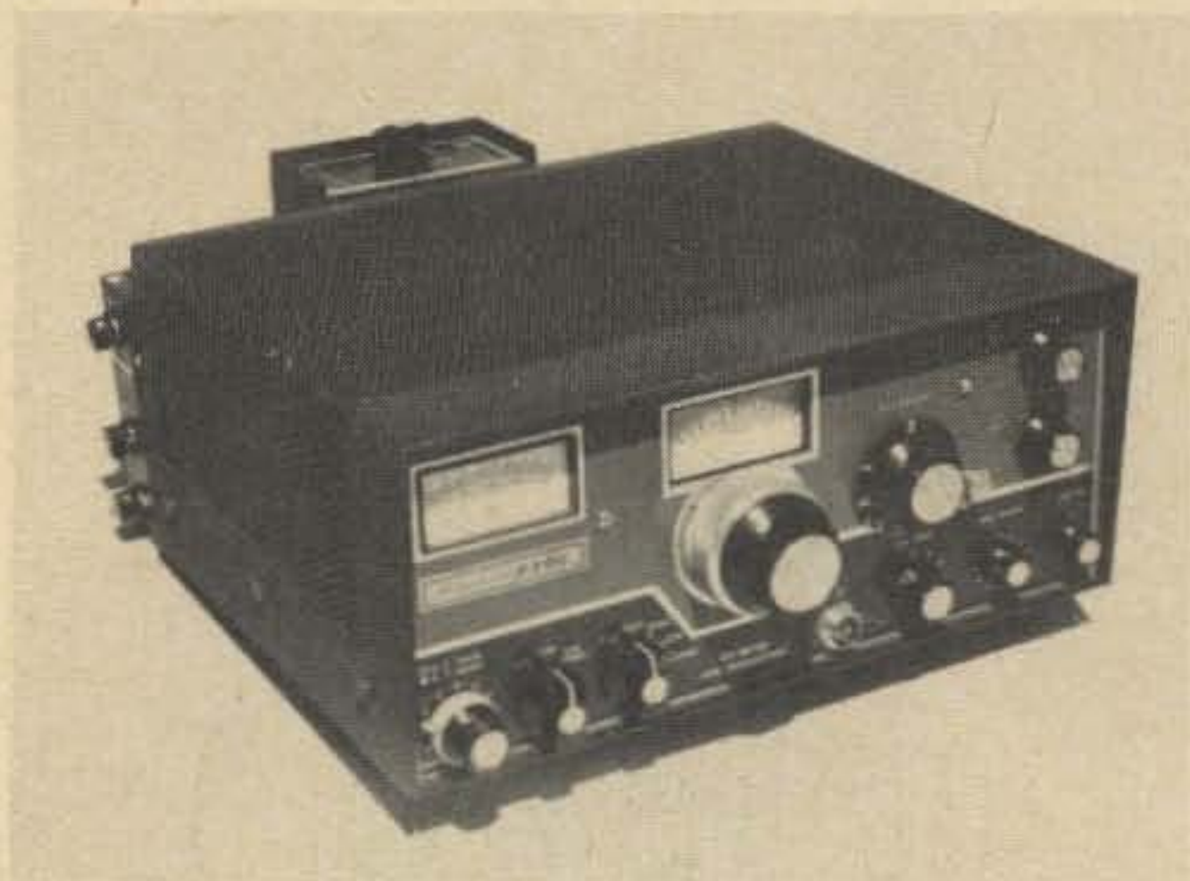
Front view of completed project. Be sure to line top of silencer with top of transceiver.
