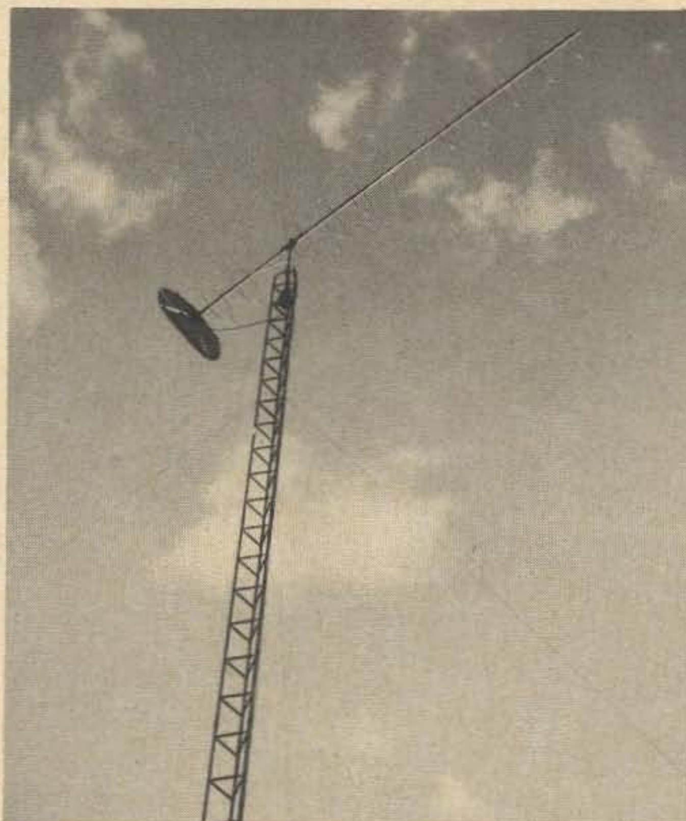
Fig. 1. This photo shows the completed 11-element 2 meter circular quad. Screen size is only 4 ft, and found to be inadequate, unless it could be increased to 200 inches. An 8 ft diameter screen reflector would have cost $48 for materials alone! Forget about "chicken wire" and you'd need a "cherry picker" for hardware cloth, because of the weight.
