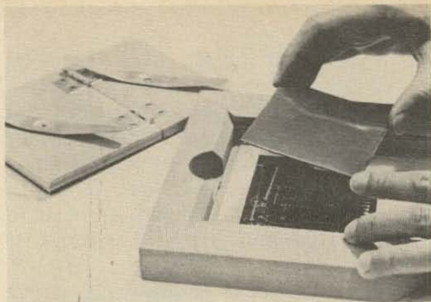
Step 5. Finished B-Neg and photoresist-coated copper-clad laminate are placed in contact frame.
