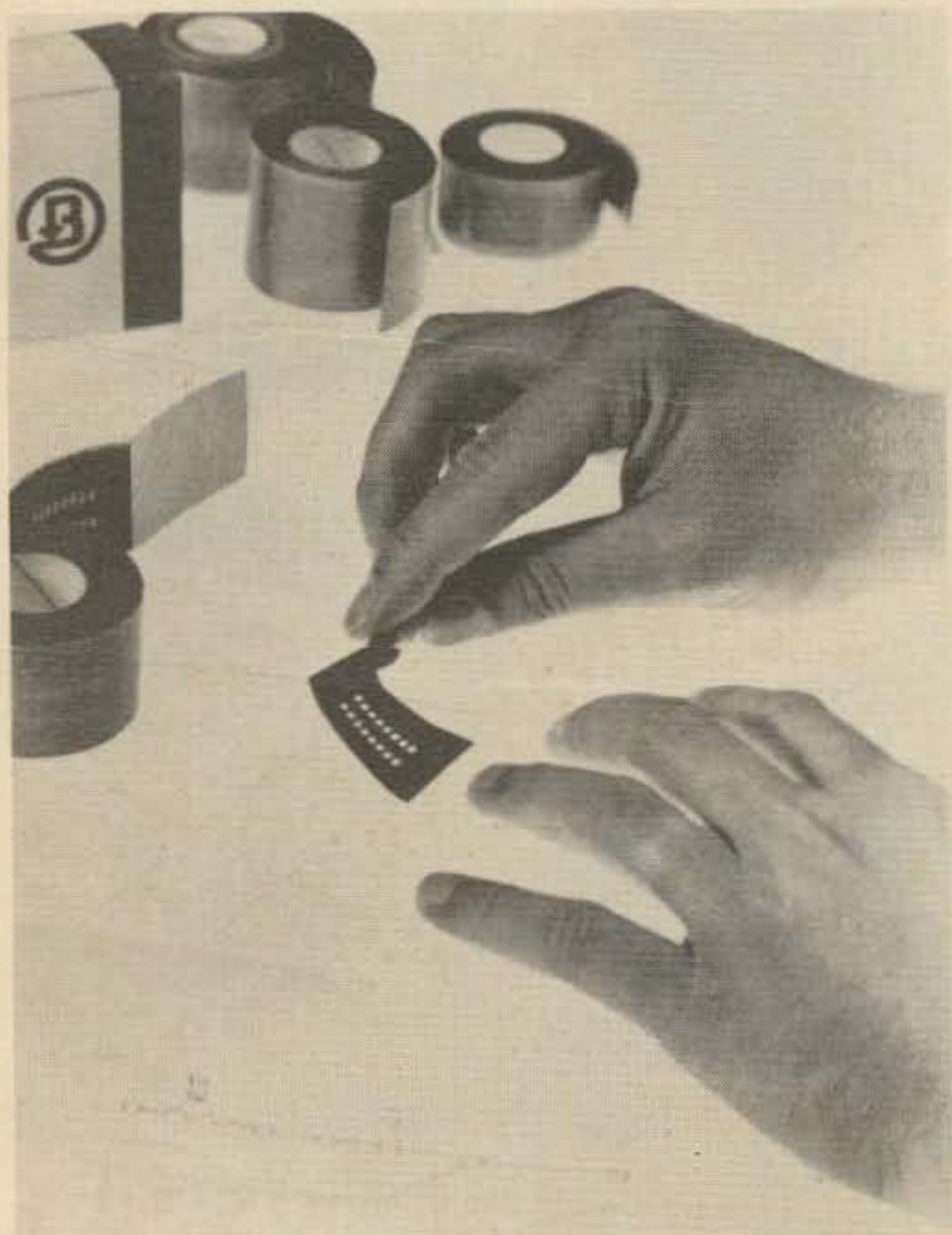
Step 1. Negative (B-Neg) version of a typical dual in-line IC package is laid down just the way positive configurations are handled.
