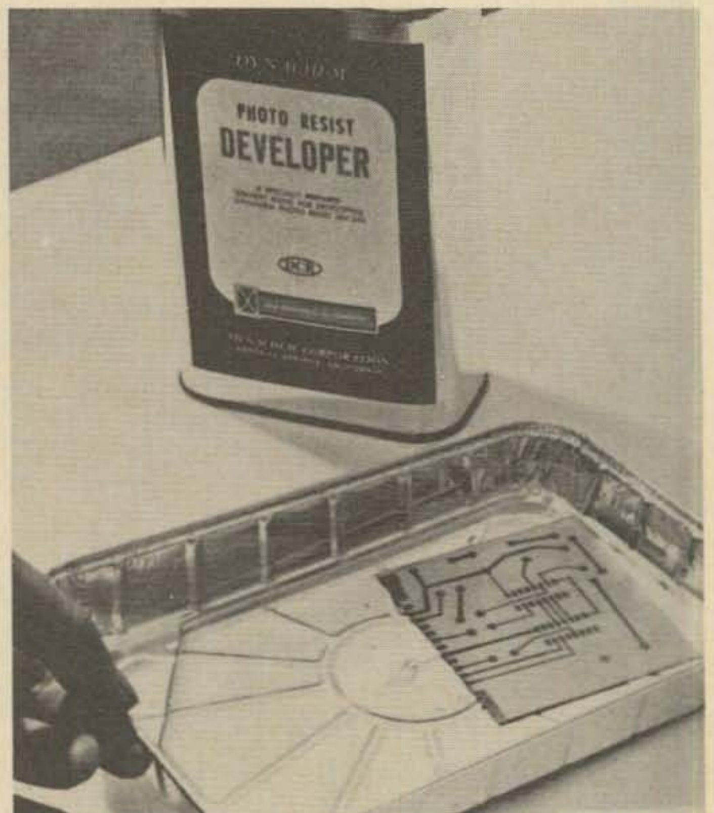
Step 7. It takes only a few seconds for a crisp pattern to show in the developer tray.
