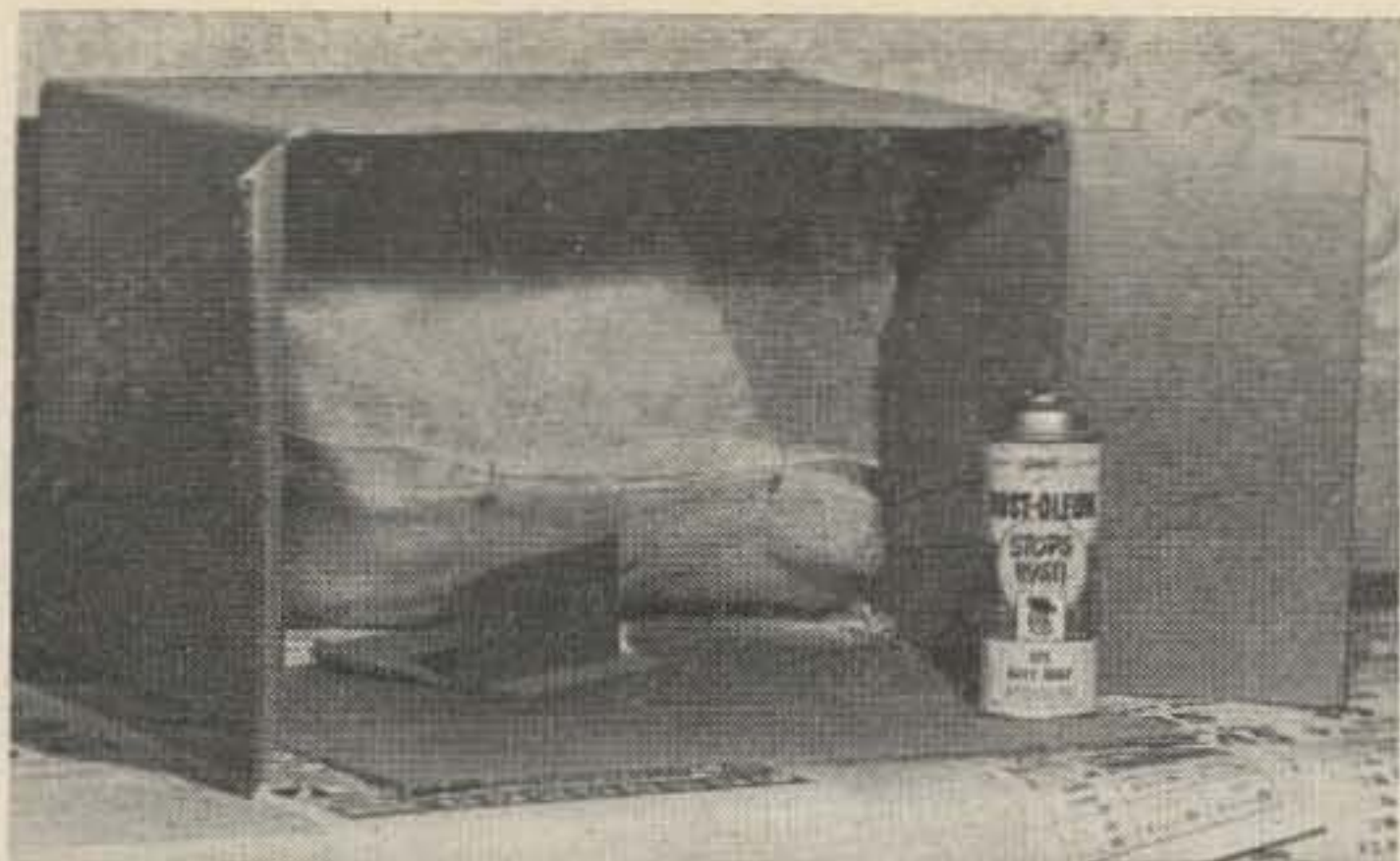
Simple spray booth. Maybe ten cents in materials. Store it front down to keep dust out.
