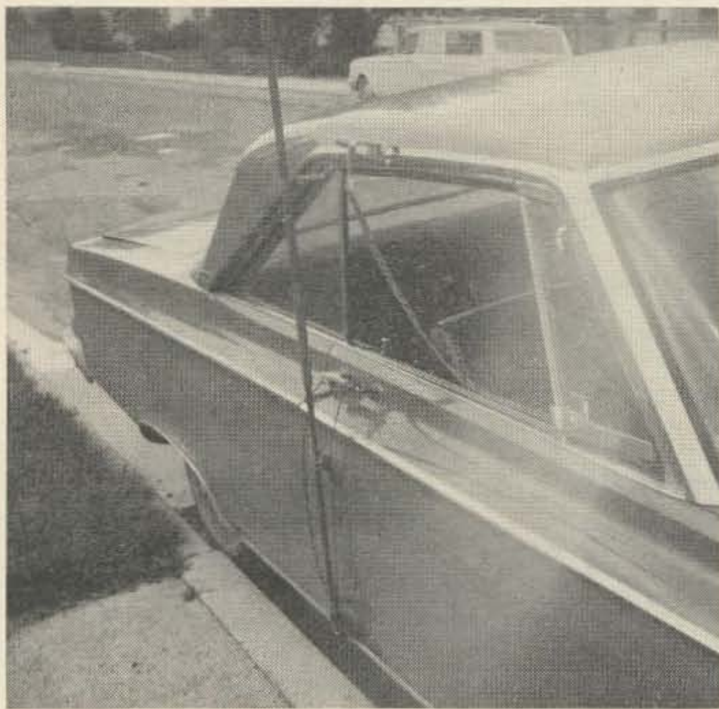
It's not very pretty, but this temporary antenna both stays on the car at 60 mph, and performs well.
