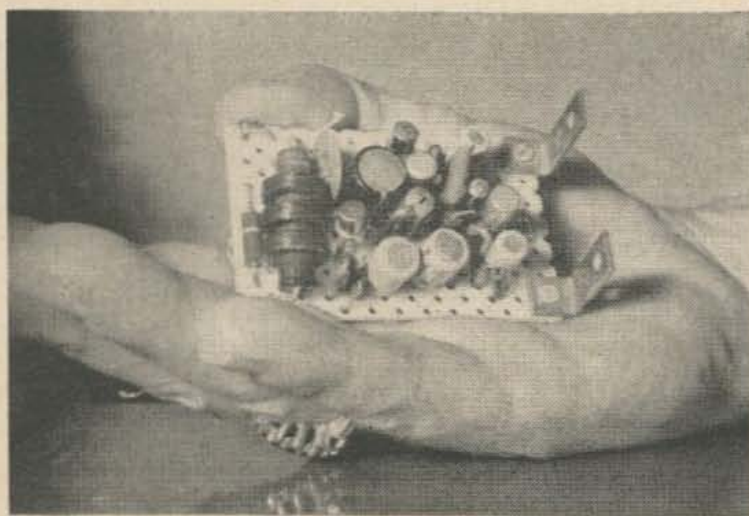
This photo shows the small size of the compressor board (1½" x 2½"). The RF filter mentioned in the text is mounted at the left.
