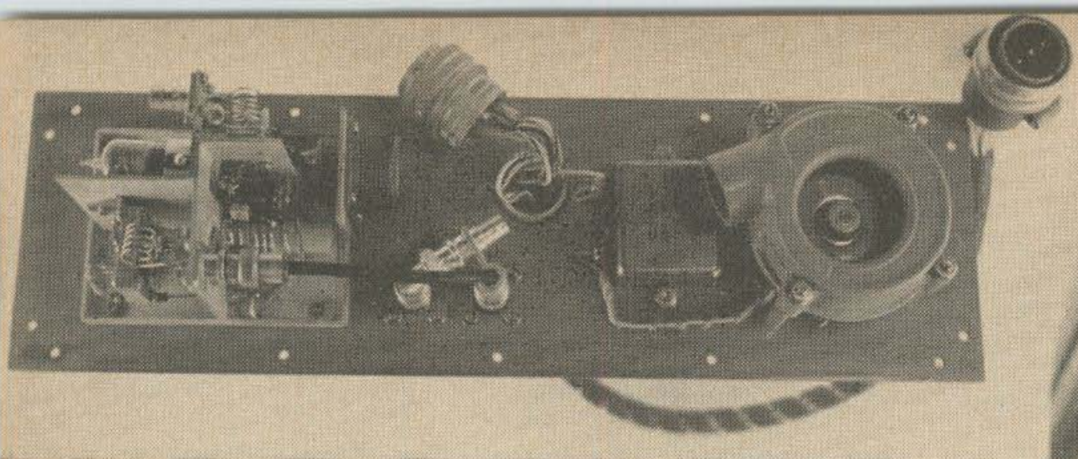
Rear of the APA-2 preamp. The blower, connectors, 6BQ7 and 416B can all be seen with the cover off.
