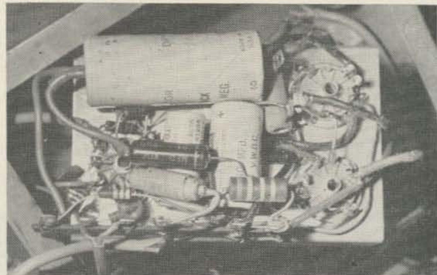
Fig. 5—Modulator Sub-Chassis: The two 6CZ5 sockets are at the left. The choke in the photo was wired in the filament lead of the 6AN8. It was later found not to be necessary, but was left in.
