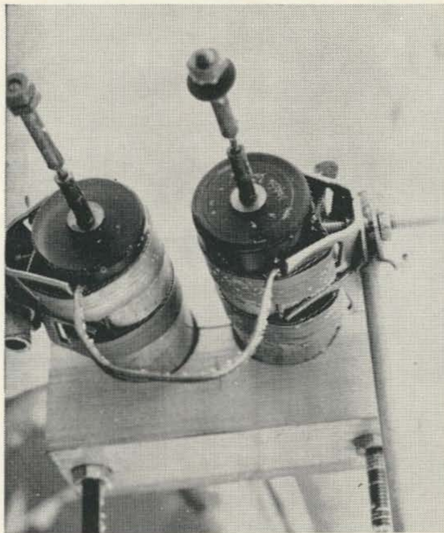
Feed point of the antenna and view of the first element and separator block.
