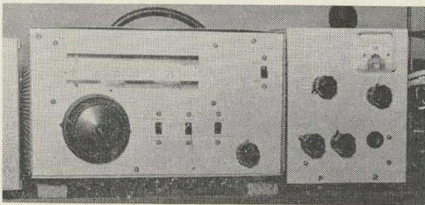
Shows the transmitter front view. The knob lower right corner is the band switch. The unit to the right is the linear amplifier.
