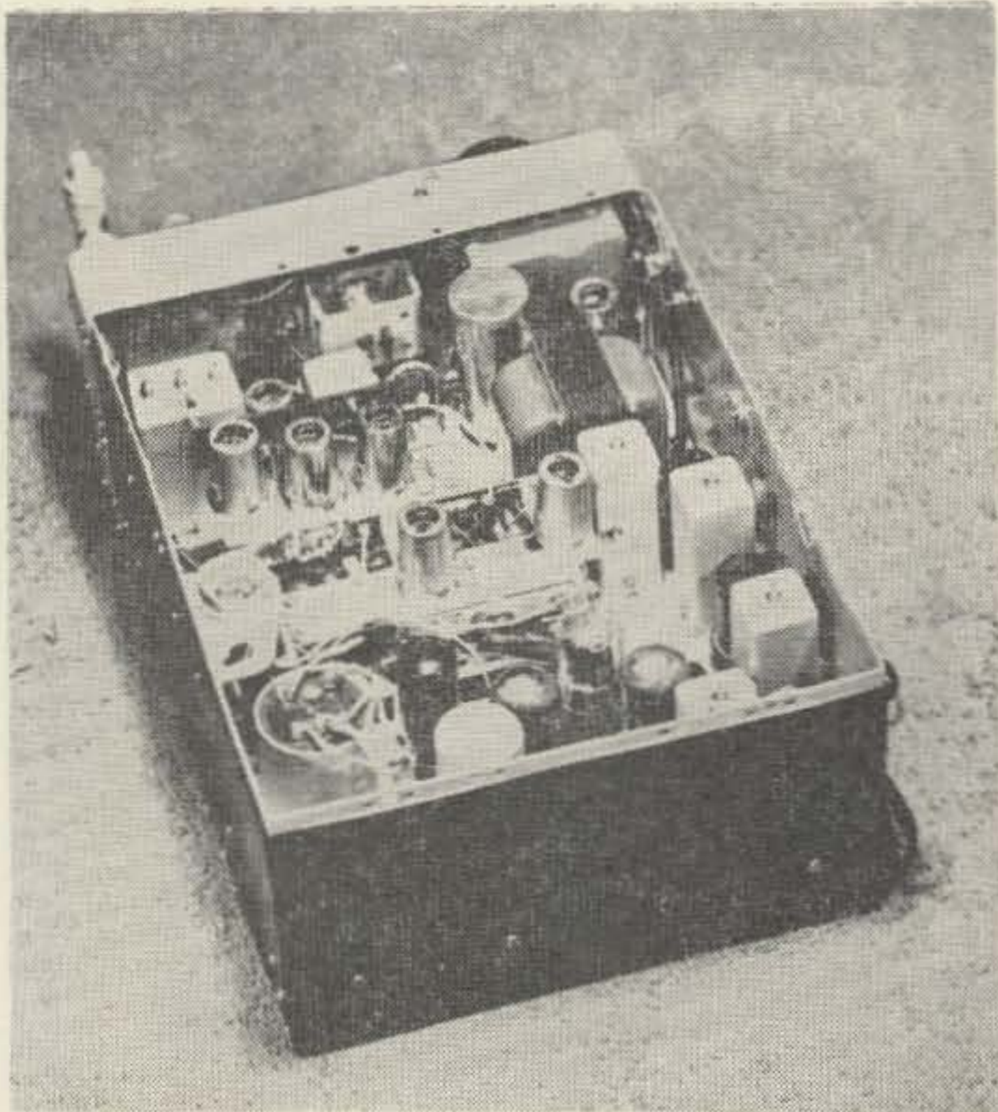
Top view of the converted receiver shows the HFO box and the speaker mounted on the front panel. Power supply components are mounted in the upper right corner of the chassis.
