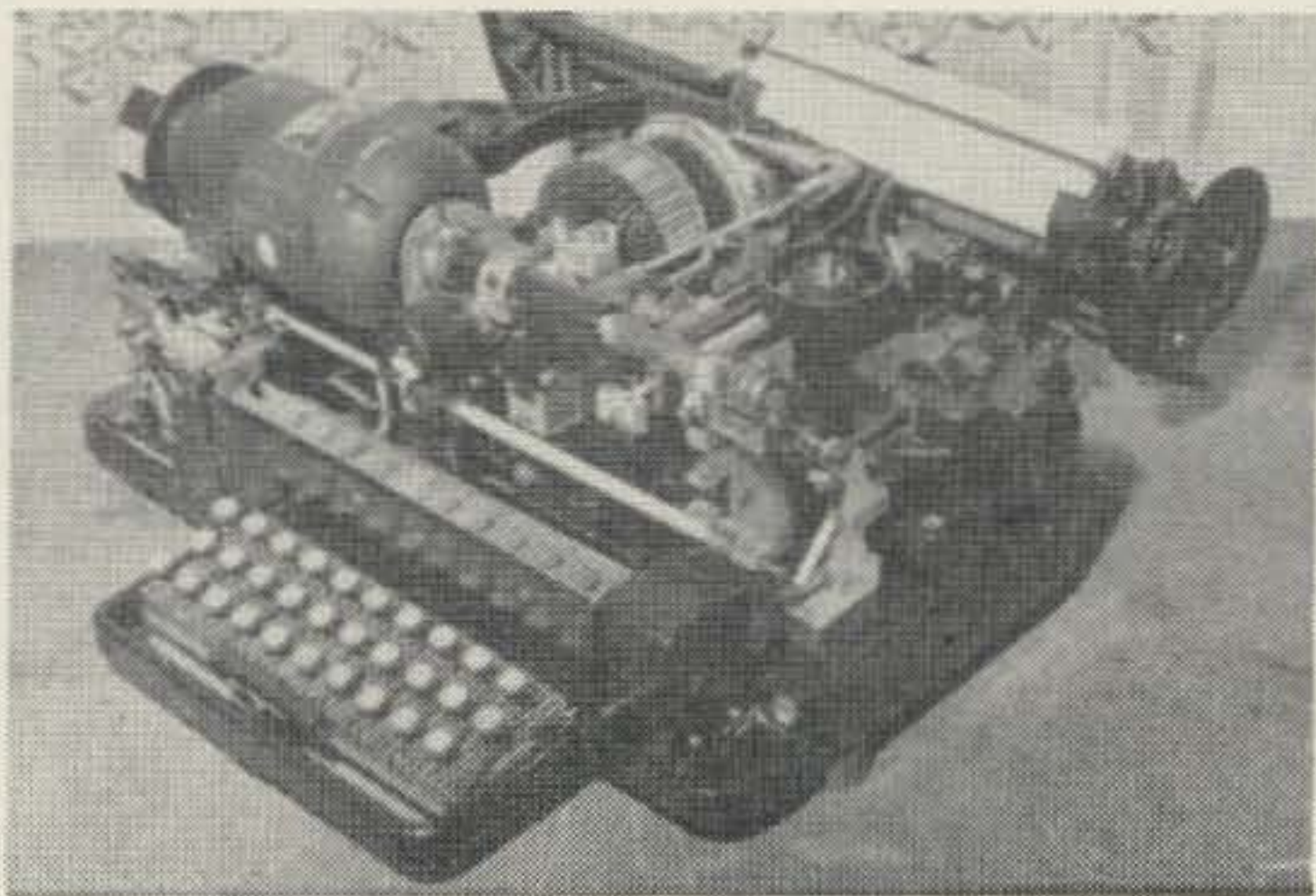
The other teleprinter used by British radio amateurs, the Creed Type 7 Page printer.
