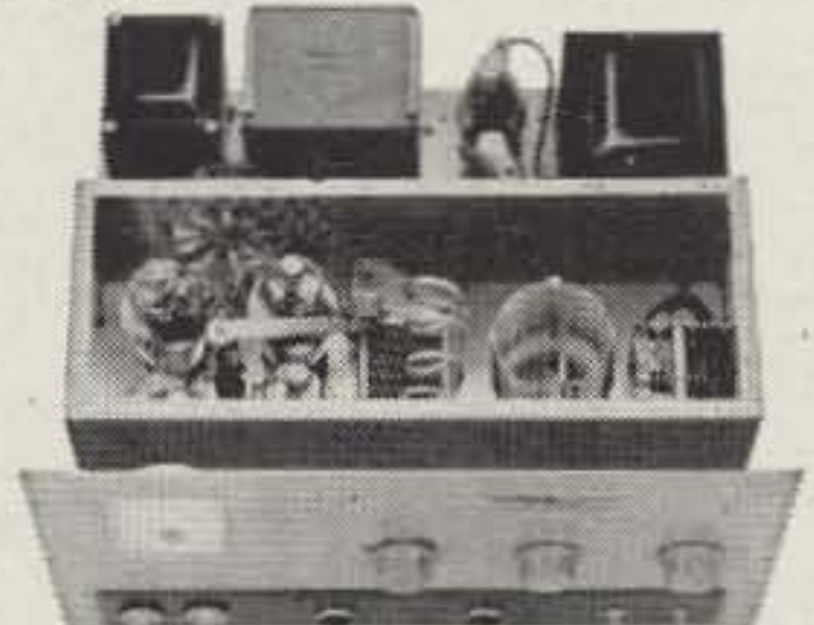
This inside view shows the neat circuit layout and husky components that emphasize quality. Note the internal shielding of plate circuit for maximum protection against TVI.
