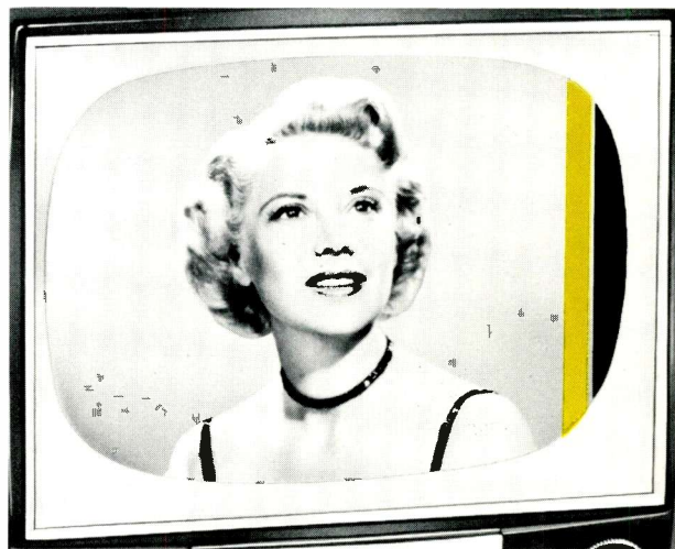
Plate 4. Appearance of the transmitted color stripe.
