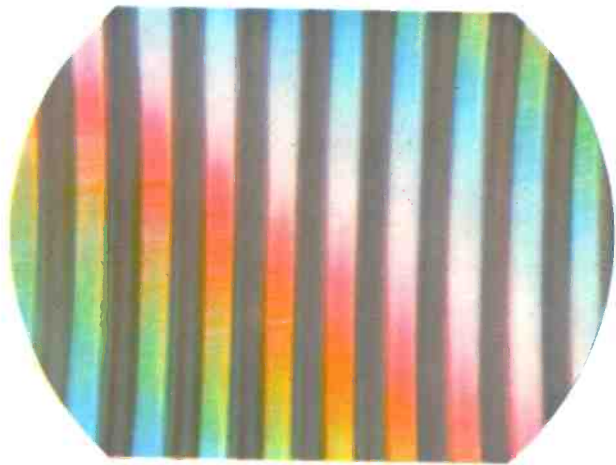
Plate 2. Loss of color sync.
