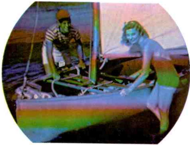
Plate 2. Loss of color sync.
