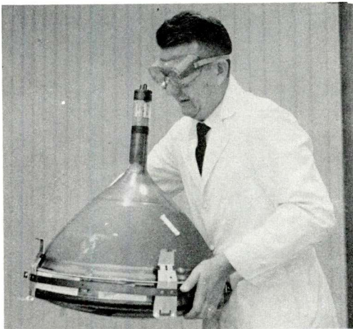
Fig. 2-41. Correct way to handle the color picture tube when installing it or removing it from the color receiver.
