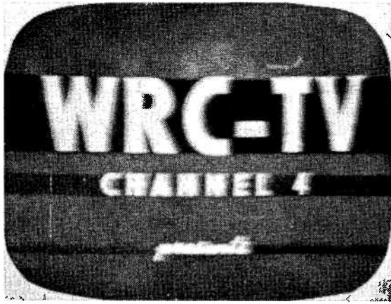
Fig. 3. Poor low-frequency response.
