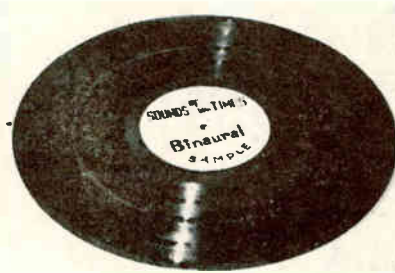
Fig. 6: Close-up of binaural recording shows the two bands of grooves
