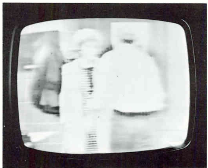
Fig. 21. Smeared video and loss of fine detail produced by shunt capacitance in the video amplifier.
