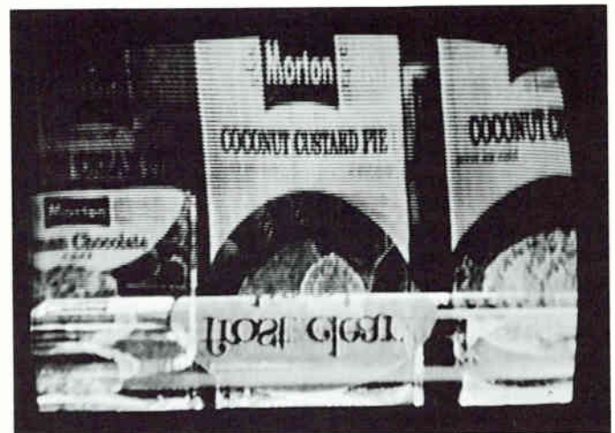
Fig. 27. Vertical foldover due to a leaky coupling capacitor on the grid of the vertical output stage. Notice the inverted lettering on the bright foldover at the bottom of the picture.
