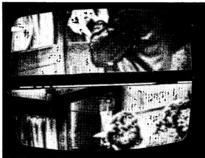
Fig. 18. Vertical blanking bar showing signals present during the vertical blanking period.
