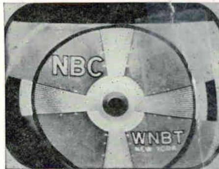
Courtesy RCA U. The lower left corner is shaded because of a misadjustment of the ion trap.
