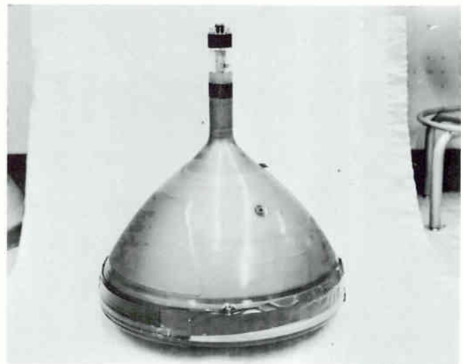
Fig. 30. 21" round picture tube resting on soft blanket.
