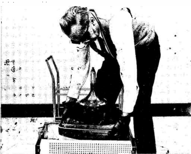
Fig. 27. Removing the picture tube from the cabinet.
