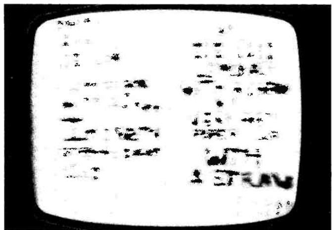
Fig. 2. The fine picture detail is missing due to poor high-frequency response.
