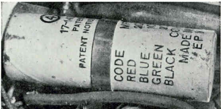
FIG. 16. Leakage may develop through the case to the strap in a condenser mounted this way.
