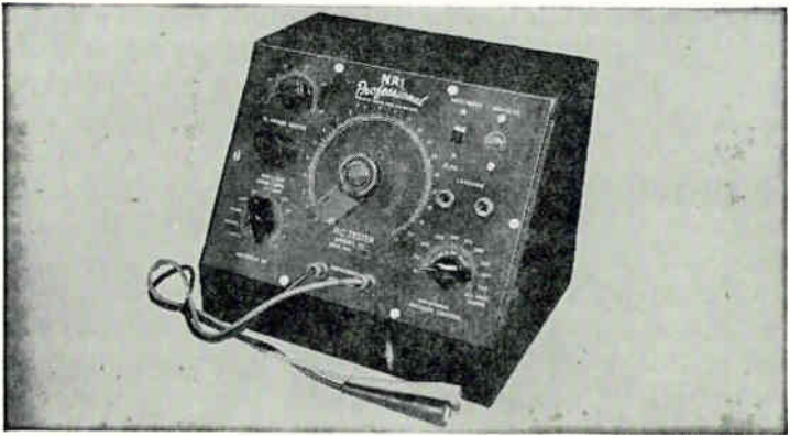
FIG. 2. The NRI Model 111 Professional R-C Tester. This instrument can check condensers for capacity, opens, shorts, leakage, and power factor. It also measures resistance. "Extra" instruments like this are time savers—worth having after a service business is established.
