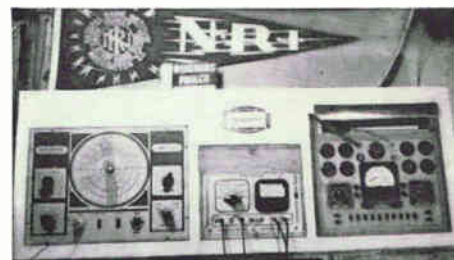
Here is Marcel Ravera's instrument panel showing the NRI Tester mounted, ready for use in Radio servicing. The NRI Tester, being a combination vacuum tube voltmeter and multimeter, often substitutes for a professional instrument with beginners. Mr. Ravera sent us this photograph.
