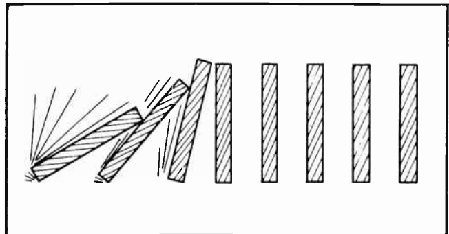
Fig. 16. The energy of the first falling domino is transmitted from one domino to another in the form of a wave. No domino moves any great distance, but the energy is quickly transmitted from the first domino to the last.
