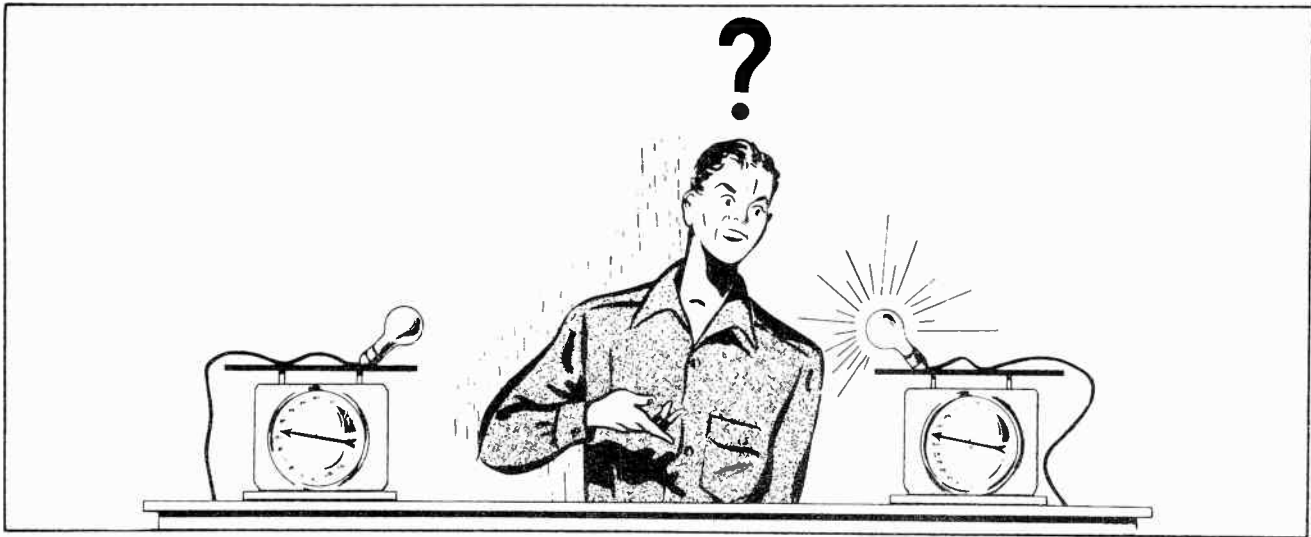
Fig.2. It is not possible to detect a passing electrical current by weighing the wires.
