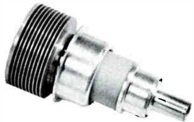
This transmitting type triode, used as a power amplifier, has an indirectly heated cathode and a metal and ceramic envelope. When forced-air cooled, its anode can dissipate up to 100 watts.
