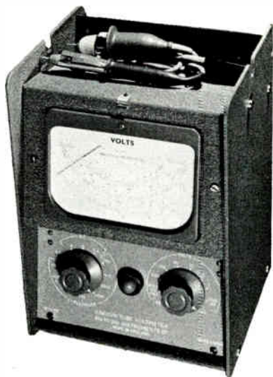
A precision VTVM featuring accurate ac voltage readings from audio to ultra-high frequencies (uhf). It measures dc voltages and a wide range of resistances. High input impedance insures very little loading of almost any ac or dc circuit.
