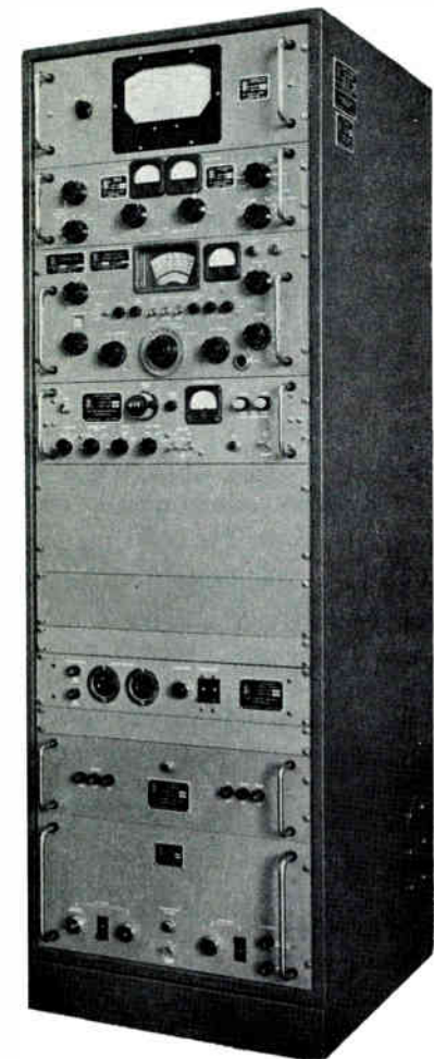
This 350 watt transmitter is built for operation in the 2 to 32 MHz range in shipboard, land and mobile installations.
