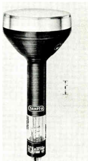
A 5 inch crt used in radar and oscilloscope applications. This tube uses electrostatic focus and electromagnetic deflection.
