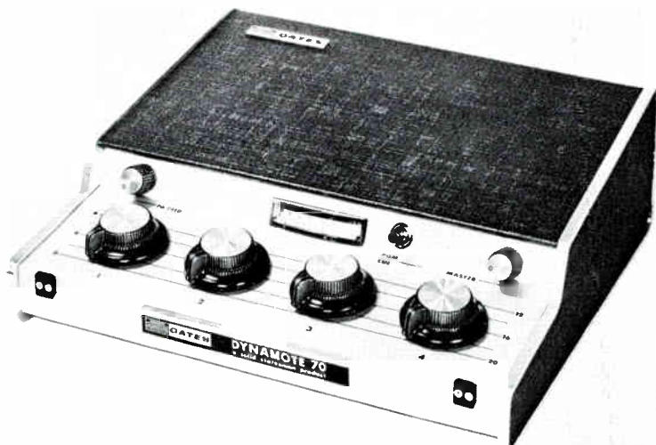
Telephone lines are used to connect this remote amplifier to the studio console. Courtesy Gates Radio Co.
