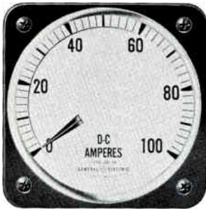
The scale of an ammeter used to measure currents from 0 to 100 amperes.
