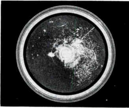
This standard radar display uses intensity modulation of the crt's electron beam to produce a map of the surrounding area. Courtesy Philca Corp.
