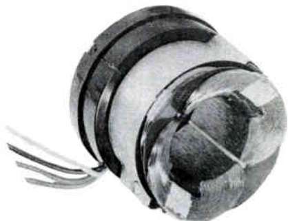
In electromagnetically deflected cathode ray tubes, the sawtooth currents in the deflection coils produce magnetic fields which move the electron beam to the proper places on the face of the crt.
