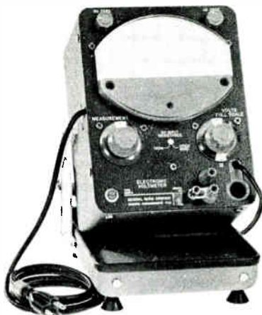
This electronic voltmeter measures dc voltages and low frequency ac voltages up to 1500 volts without the use of external multipliers. Its ohmmeter range is from .2 ohm to 1000 meg-ohms.
