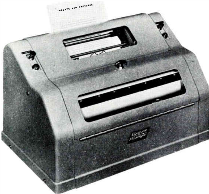
A facsimile transmitter for sending maps, sketches, written or printed matter from one city to another via microwave, telephone, or private lines.
