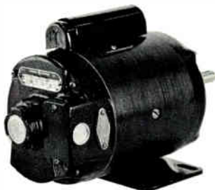
Resembling a motor, this device is an electric generator capable of producing 115 volts dc at approximately 4.4 amps. Thus, the power capability is about 500 watts.
