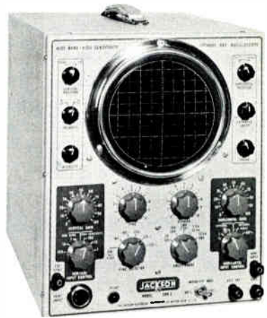
This wide band, high sensitivity scope has a vertical attenuator plus vertical gain control to attenuate the vertical input signal.
