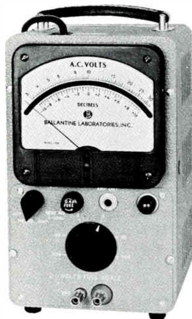
A general purpose electronic voltmeter for precision measurement of ac voltages.
