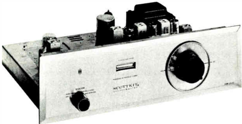
A full wave vacuum tube power supply is used in the stereophonic FM tuner shown above. The power transformer is the large black object at the rear of the chassis.
