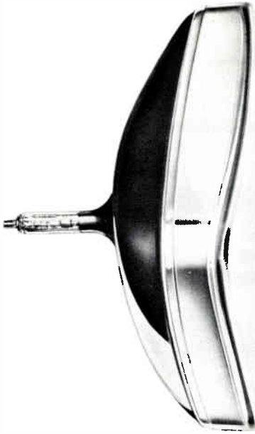
The background brightness of the picture tube screen is determined by the bias applied between its grid and cathode.
