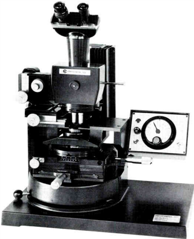
The split-field microscope and exposure system shown above is used for split-field viewing and rapid aligning and exposure of sequential patterns. It provides magnifications from 19X to 1100X.
