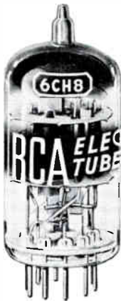
A combination tube, including a medium- \mu triode and a sharp-cutoff pentode in the same envelope.
