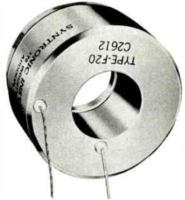
Focus coils are made to be mounted around the neck of a crt.
