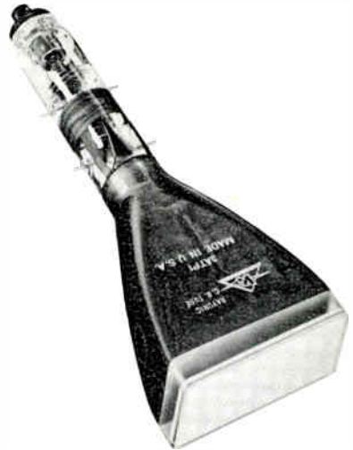
A crt with a rectangular screen used in oscilloscopes and other test equipment. This tube uses electrostatic deflection and focusing.
