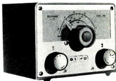
This variable frequency oscillator, VFO, is used to generate the carrier signals for an amateur radio transmitter. High frequency stability is obtained by careful construction techniques, high quality components, and the use of temperature compensating components. Courtesy National Radio Company, Inc.
