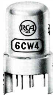
A nuvistor triode commonly used in television and FM radio tuners.
