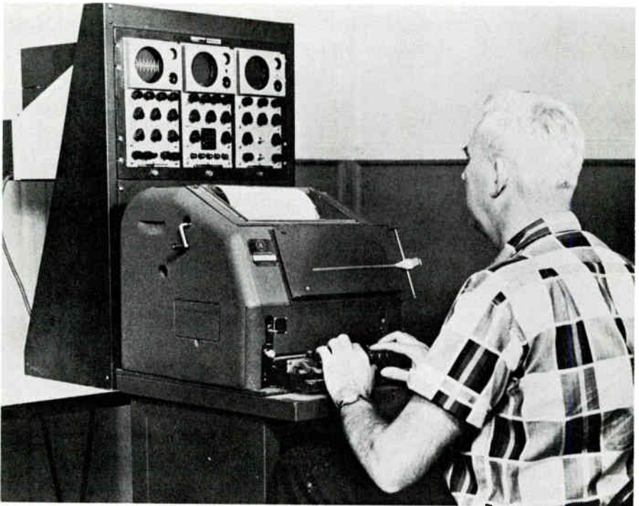
The above equipment uses special oscilloscopes to check pulse waveforms. Courtesy Radiation, Inc.
