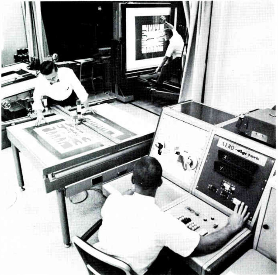
The central console shown at the right directs the passage of a razor-like blade through the masking material. This automatic process is completed in approximately 10 minutes.
