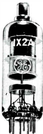
The type 1X2 diode rectifies pulses in high voltage supply circuits.
