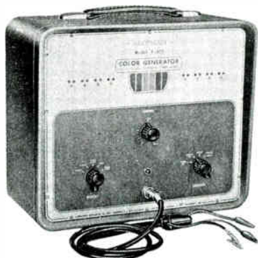
A signal generator of this type is used to align and troubleshoot color television receivers. To make use of its signals, the generator output terminals are connected in parallel with the antenna input terminals of the receiver.
