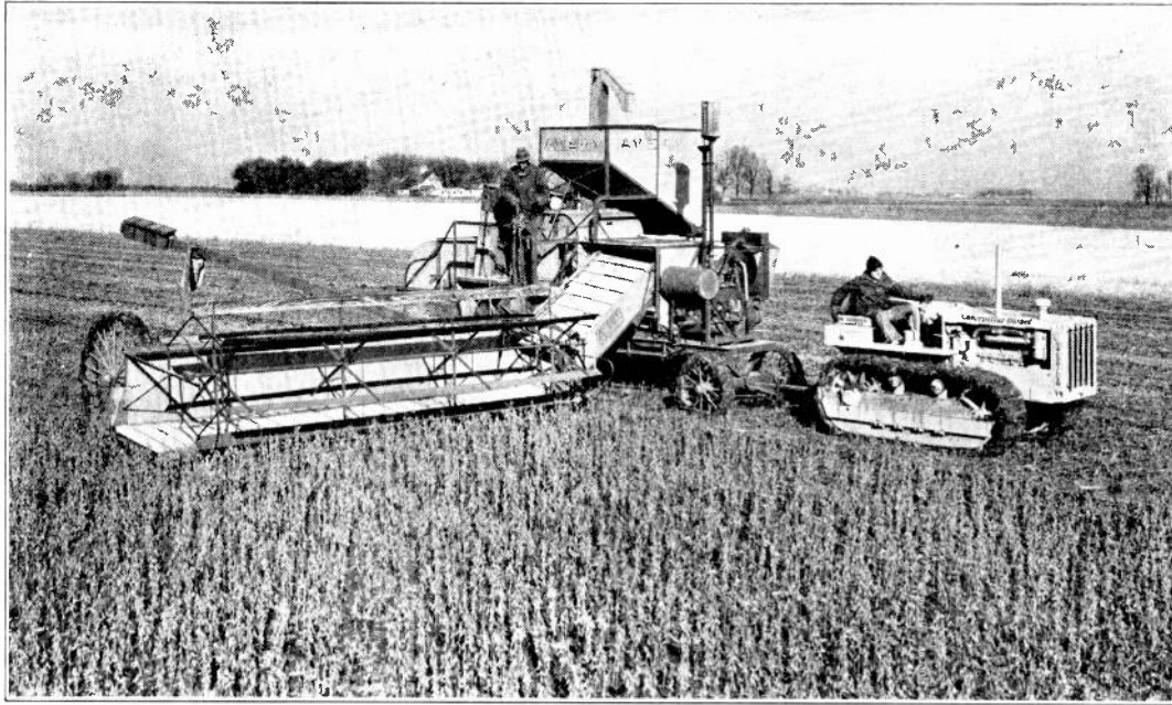
Fig. 55. This photo shows a Caterpillar Diesel tractor pulling a 16 foot combine machine harvesting soy beans. Thousands of tractors of this type are now used in farm work.
