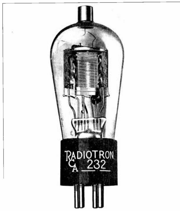
Fig. 77. This excellent photograph shows a vacuum tube with part of the outer screen grid and part of the plate removed, to clearly show the inner screen grid in its position between the control grid and plate. (Photo courtesy of R. C. A. Radiotron Co., Inc.)
