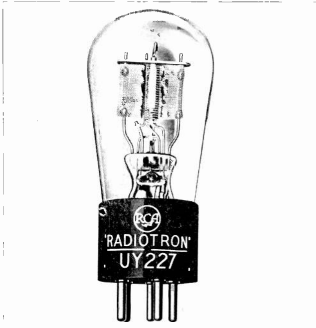
Fig. 80. Photograph of an A. C. heater-element vacuum tube with part of the plate removed to show the grid and the cathode inside of which the heater element or filament, is located. (Photo courtesy of R. C. A. Radiotron Co., Inc.)
