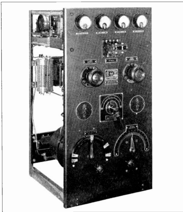
Fig. 272. Front view of a marine type vacuum tube transmitter for use on ships for communication and distress signal uses. Vacuum tube transmitters of this type are rapidly replacing all spark transmitters. (Photo courtesy of Radiomarine Corp. of America.)
