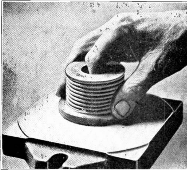
Fig. 98. The above photo shows how to hold a bellows type shaft seal on the lapping block for lapping or polishing the face of the seal. Courtesy Servel Manufacturing Company.
