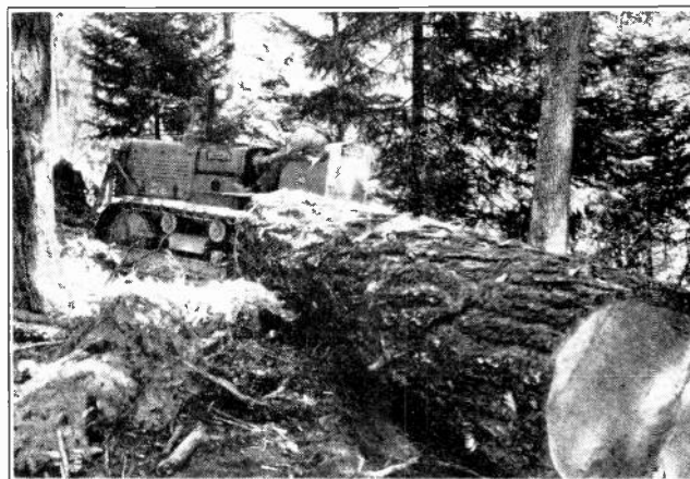
Fig. 25. This photo shows a Diesel-tractor used for dragging out logs in the lumber woods. (Courtesy of the International Harvester Company.)
