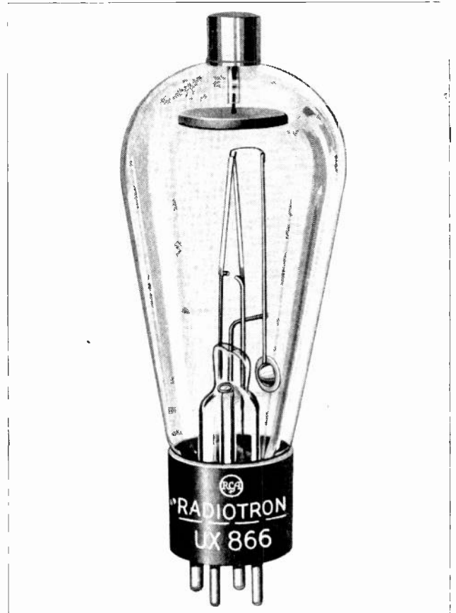
Fig. 90. Another type of half-wave rectifier tube for use with higher voltages such as required for the plates of power output tube. Courtesy R. C. A. Radiotron Company, Inc.
