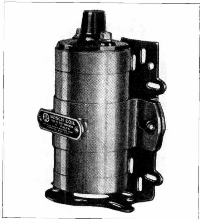
Fig. 22. High-tension ignition coil such as used for supplying high voltage impulses to the spark plugs on the ignition systems of automobiles. The heavily insulated bushing on the top of the coil is where the high voltage lead connects.
