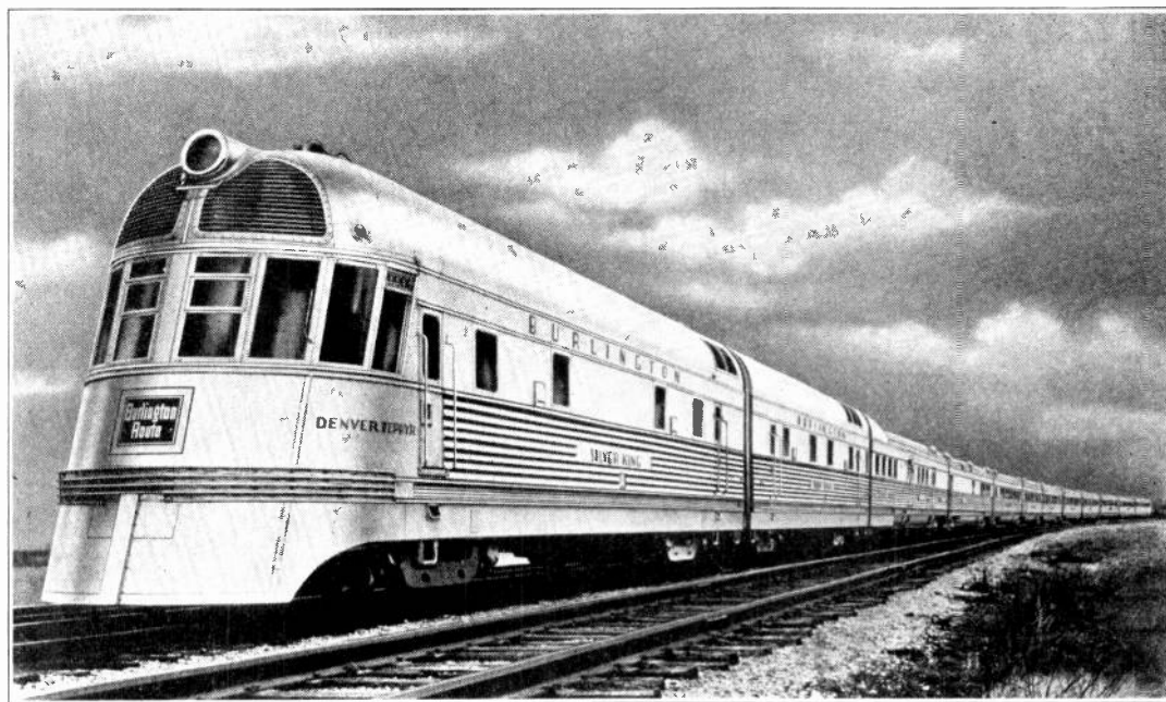
Fig. 24. Powerful Diesel-Electric generating units are becoming extensively used for operation of modern high speed trains such as shown in the photo on the right. Courtesy of the Burlington Ry.
