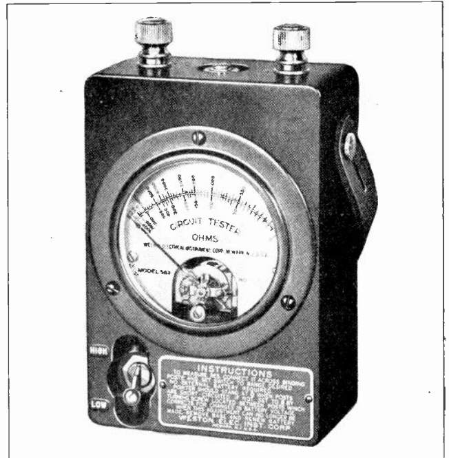
Fig. 197. Convenient Ohmmeter or circuit tester which is also very valuable for continuity testing and radio trouble shooting. (Photo courtesy of Weston Electrical Instrument Co.)
