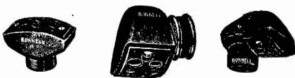
Fig. 138. Weather head fittings of the types shown above are used on the end of conduit at the service entrance to prevent water from entering the conduit.
