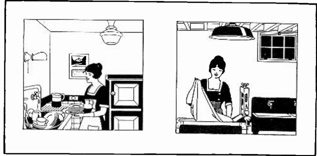
Fig. 253. At the left is shown the arrangement of ceiling unit and wall bracket light for kitchen. On the right a very efficient type of reflector for laundry rooms and basement lighting.
