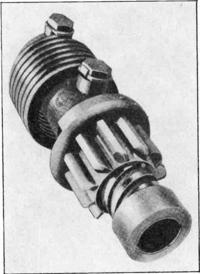
Fig. 5. Photograph view of Bendix drive mechanism showing spring, sleeve, and pinion.
