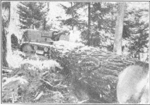
Fig. 23. This photo shows a Diesel-tractor used for dragging out logs in the lumber woods. (Courtesy of the International Harvester Company.)
