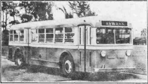
Fig. 12. This view shows a modern motor bus equipped with a Diesel-Electric drive unit such as shown in Fig. 12A. (Courtesy of the Hercules Engine Company.)
