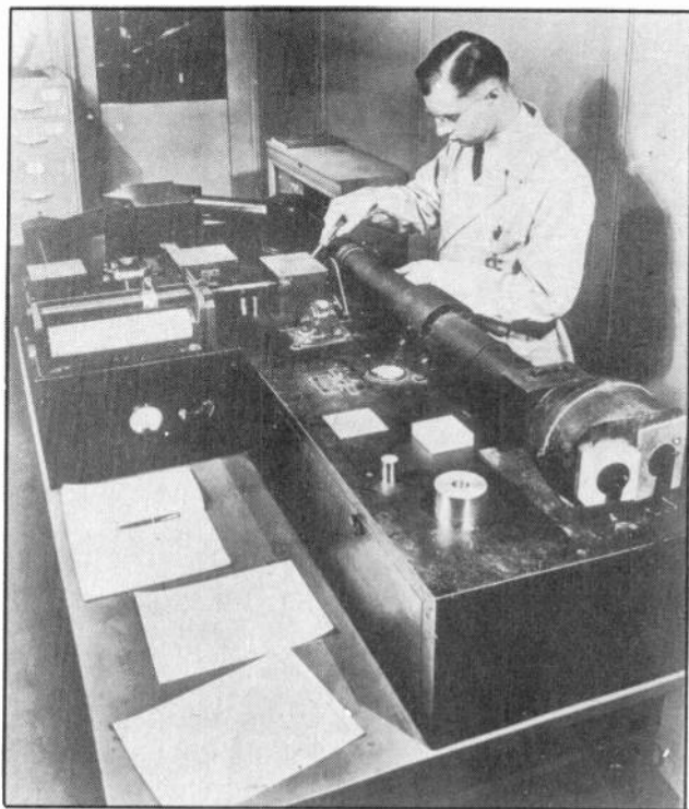
A recording spectrophotometer, a high-precision Electronic instrument widely used in the paper, textile, chemical, and paint industries for analyzing.
