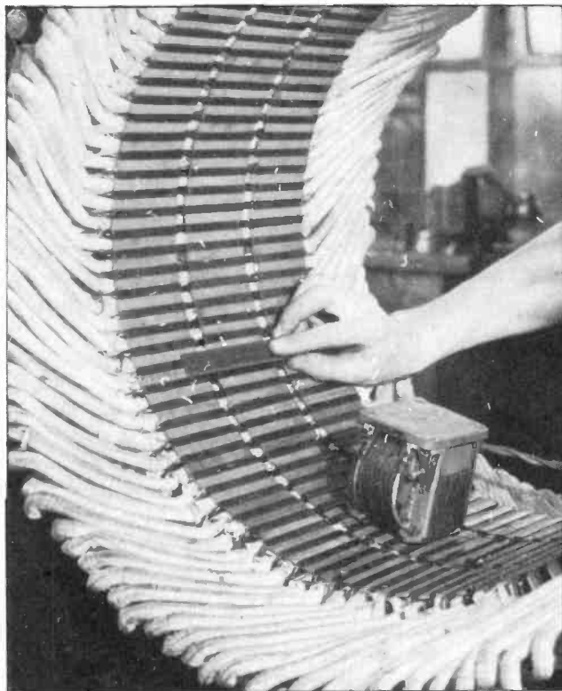
Fig. 9. This photo shows a growler in use in a large stator. Note the size and shape of these coils and the position of the steel strip which is just the width of one coil from the center of the growler.
