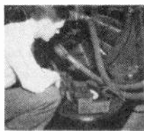
Fig. 2.C DON'T use instruments near strong fields such as the cables shown here which are connected to a generator.
