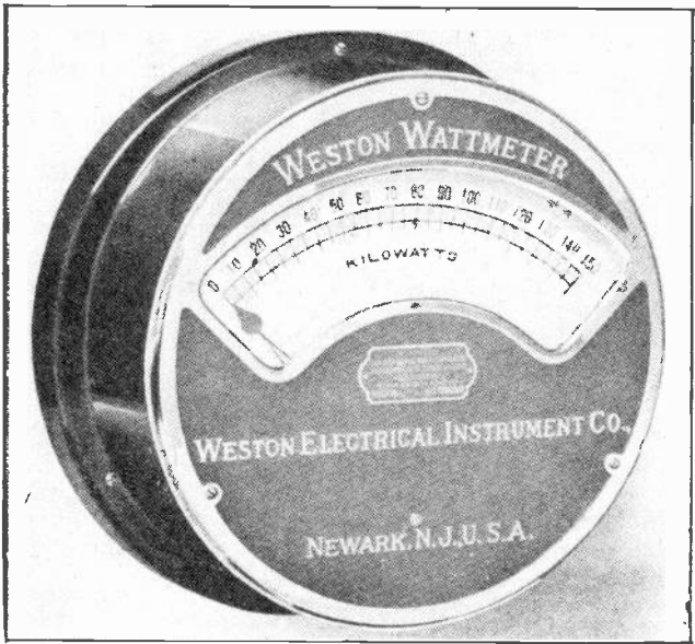
Fig. 12. Switchboard type wattmeter which has its scale calibrated to indicate the load in kilowatts. (Photo courtesy Weston Electrical Instrument Co.)
