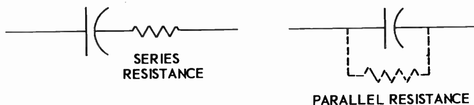
Fig. 29-4. Energy losses in capacitors may be represented as equivalent resistances.
