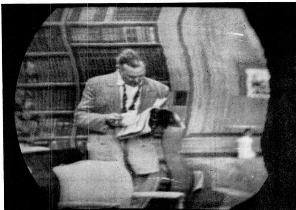
Fig. 93-7. Severe bending or pulling extending all the way from top to bottom of the picture. This picture has been moved to the left in order to show bending of the right-hand edge, which would show up also on a raster.
