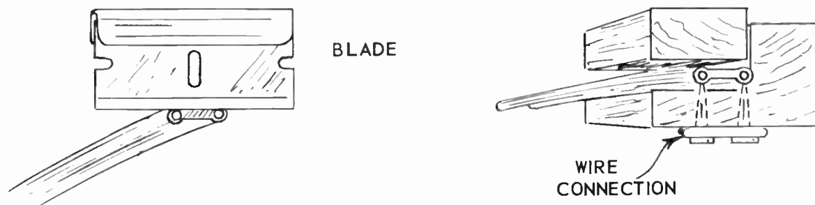
Fig. 68-14. Methods of temporarily short circuiting a stub at various points along its length.
