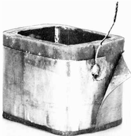
Fig. 77-6. An electrostatic shield around the outside of the primary winding in a power transformer.
