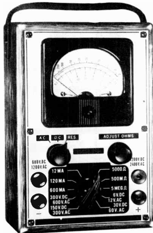
Fig. 71-9. A multi-range volt-ohm-milliammeter.
