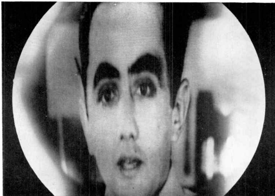
Fig. 93-12. Vertical non-linearity most often causes stretching at the top of pictures. Horizontal trace lines then are farther apart at the top than lower down.
