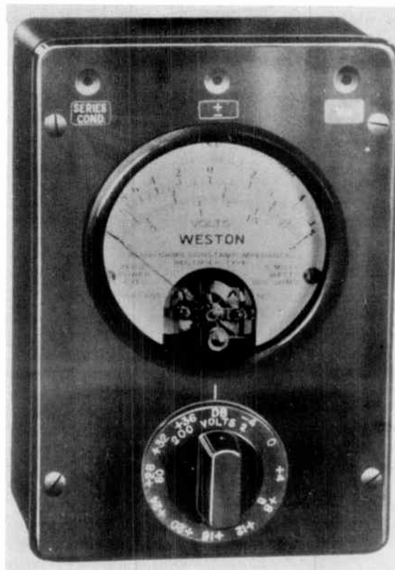
Fig. 39-9. Output meter for measuring voltages at audio frequencies.
