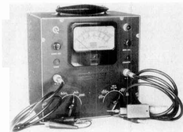
Fig. 39-7. Service type electronic voltmeter.
