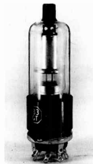
Fig. 62-11. A 1B3-GT high-voltage half-wave rectifier tube.
