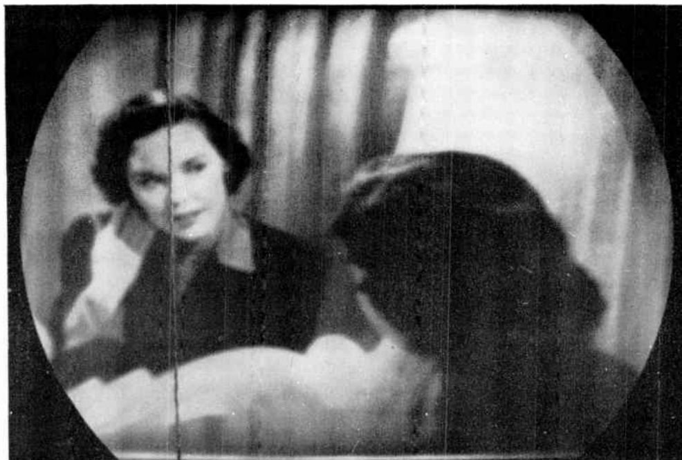
Fig. 94-7. A dark, or dark and light, vertical line at the left indicates Barkhausen oscillation.
