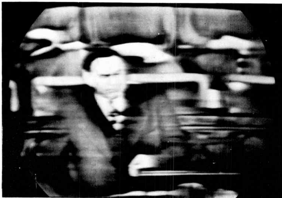
Fig. 93-4. Smears or trailers. This picture shows an extremely bad condition. Even slight smearing causes unsatisfactory reproduction.
