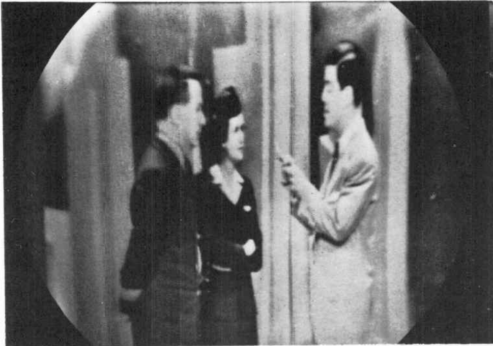
Fig. 93-10. Horizontal non-linearity here is causing compression at the center of the picture area.
