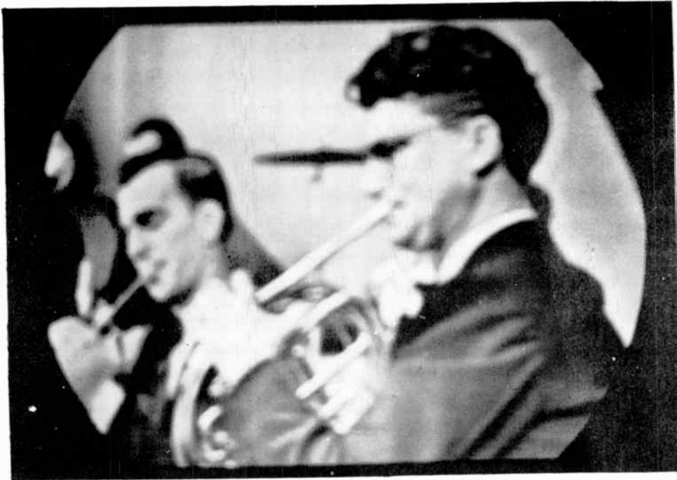
Fig. 93-1. Focus incorrect. The appearance here is not due to poor resolution, but to an electron beam spot which is too large to form distinct horizontal trace lines.
