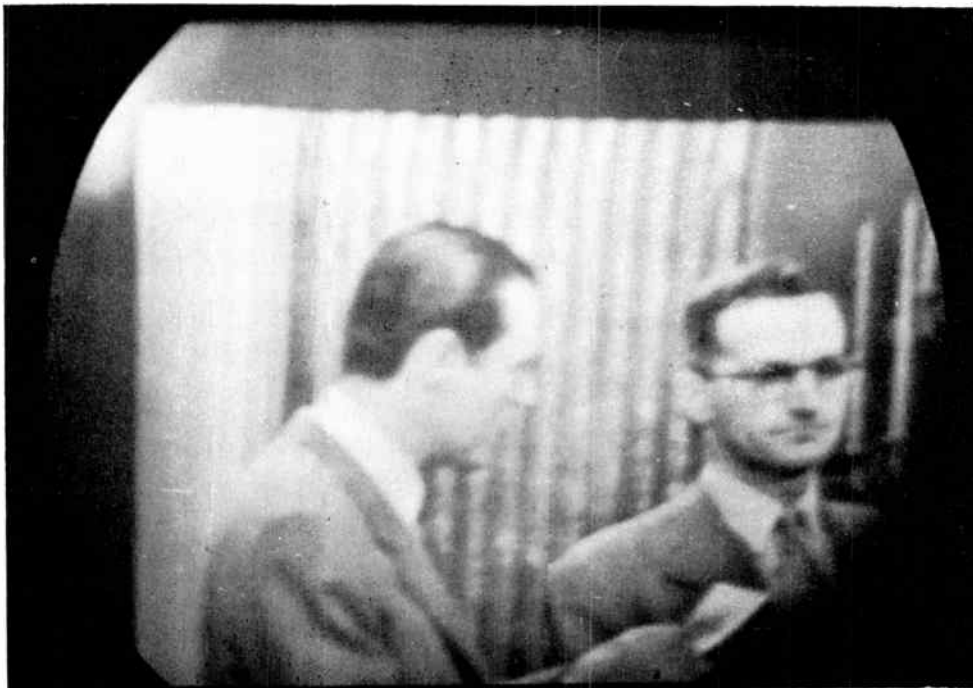
Fig. 93-8. This picture is off center toward the right and toward the bottom. Centering may be faulty in any direction, upward, downward, or toward either side.
