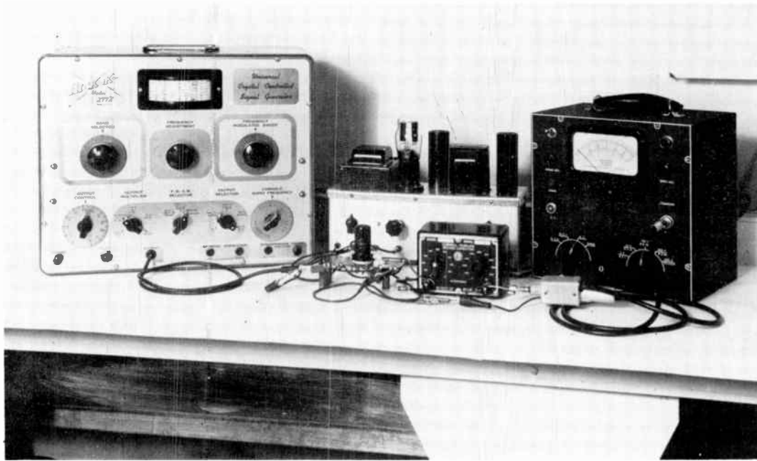
Fig. 47-5. Test setup for checking the effect of coupling capacitors on gain at various frequencies.
