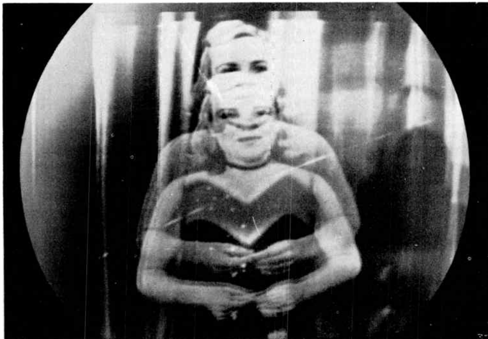
Fig. 93-23. Vertical sync not holding. The picture moves either upward or downward, steadily or in successive jumps.
