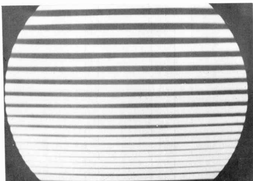
Fig. 94-24. Vertical non-linearity as shown by a bar pattern.
