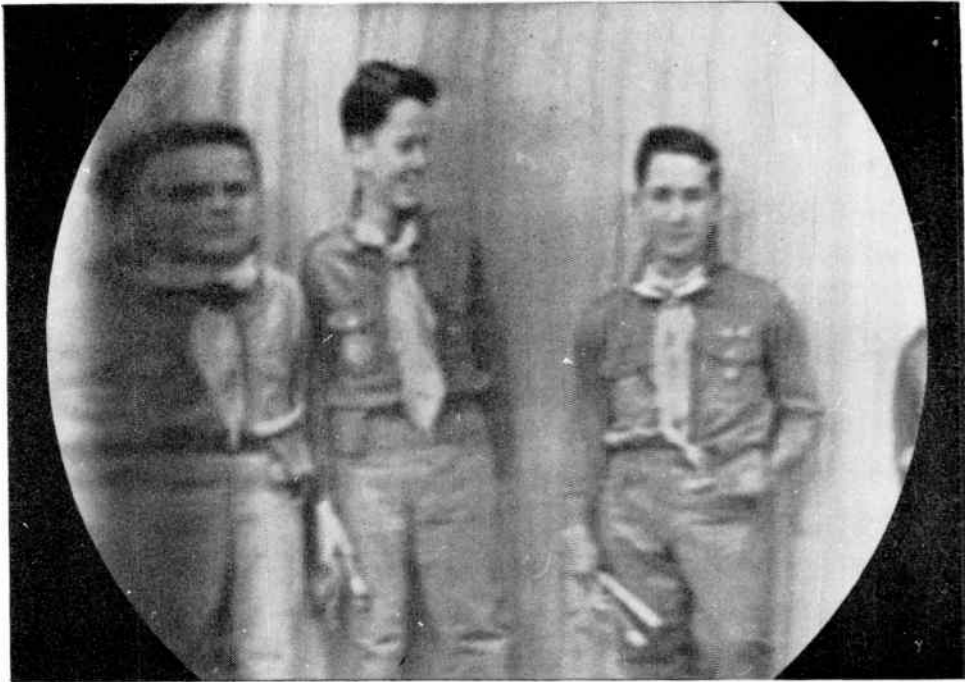
Fig. 94-6. There is a dark vertical band at the left. Note that this side of the picture is stretched, indicating too rapid travel of the electron beam where illumination is low.
