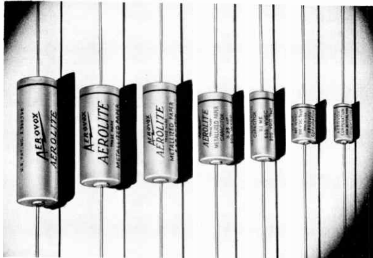
Fig. 12-3. Fixed capacitors made with paper dielectric.
