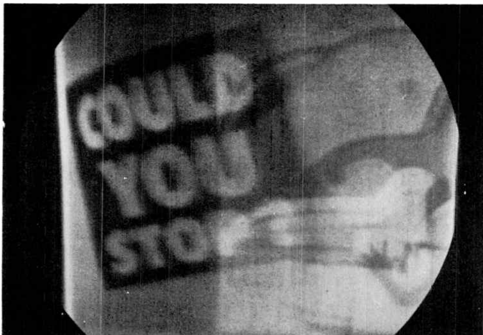
Fig. 94-12. Folded picture, horizontally. The part of the image which is stretched horizontally, is at the left in this particular case. It might be at the right.
