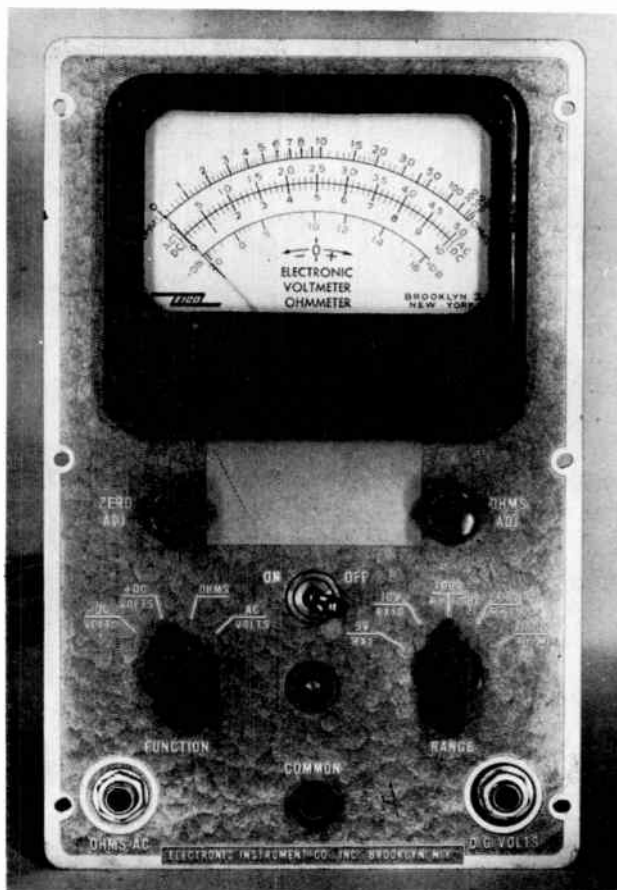
Fig. 73-7. A multi-range vacuum tube volt-ohmmeter.
