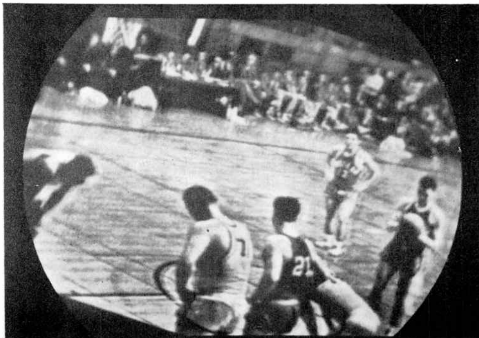
Fig. 93-18. Tilting of the picture within the mask.
