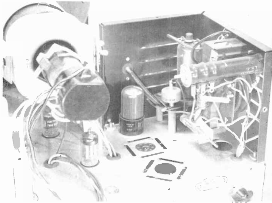
Fig. 42-14. Some of the parts in a high-voltage power supply.
