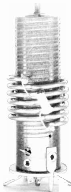
Fig. 46-11. The large winding with its connected capacitor is a trap circuit.
