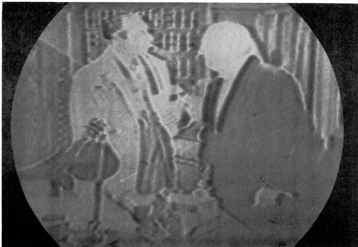
Fig. 92-12 A negative picture has generally “flat” tones, with actual or apparent interchanging of light and dark tones.
