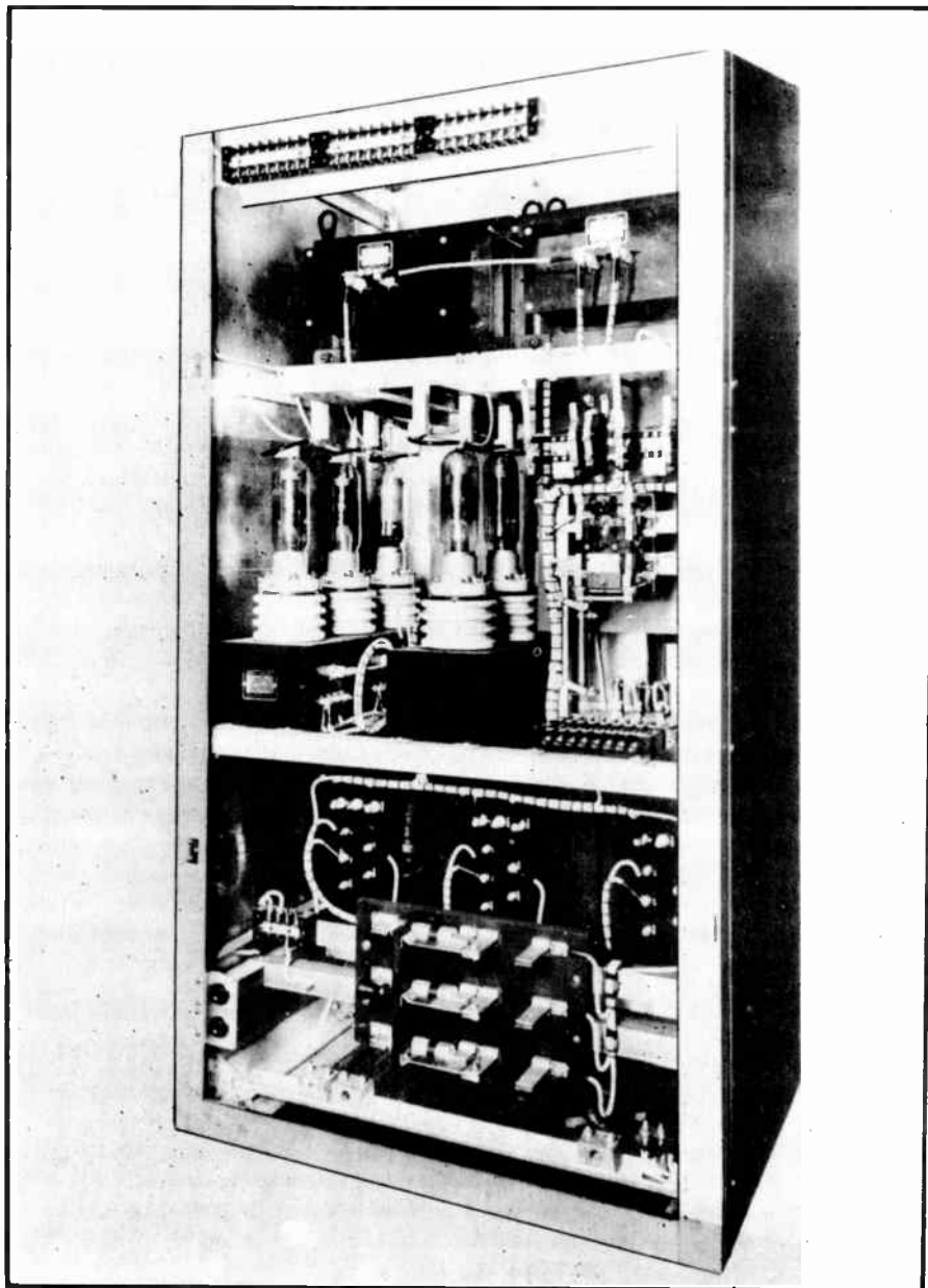
Fig. 5-1. Heavy-duty rectifiers in the modulator power supply of a television transmitter.
