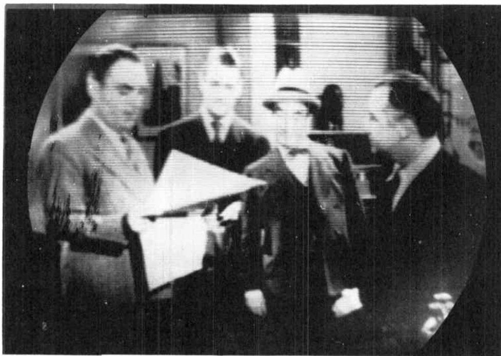
Fig. 93-2. Interlacing faulty. Note the fine horizontal lines which show up most clearly along the top of the picture.
