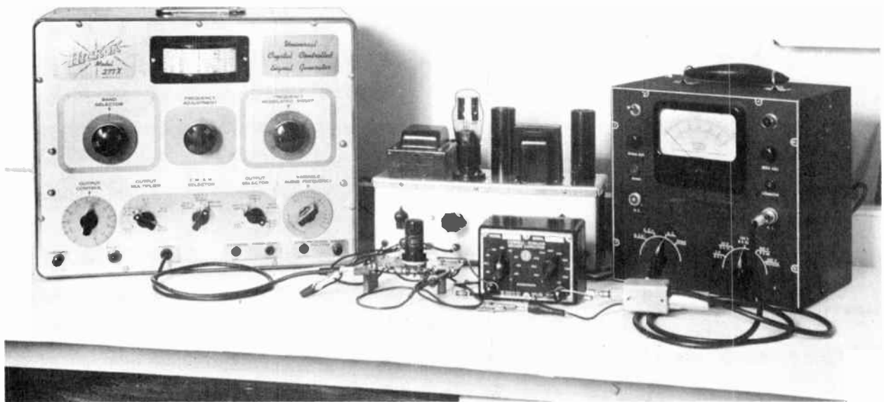
Fig. 8-1. A test setup for checking effects of different capacitors in an amplifying stage.
