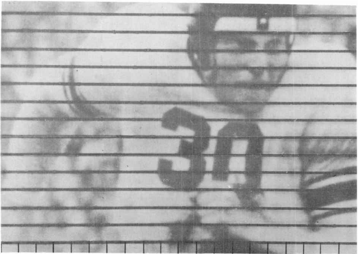
Fig. 1-8. Every horizontal line, or part of a line, consists of areas in which there is predominantly a single shade.
