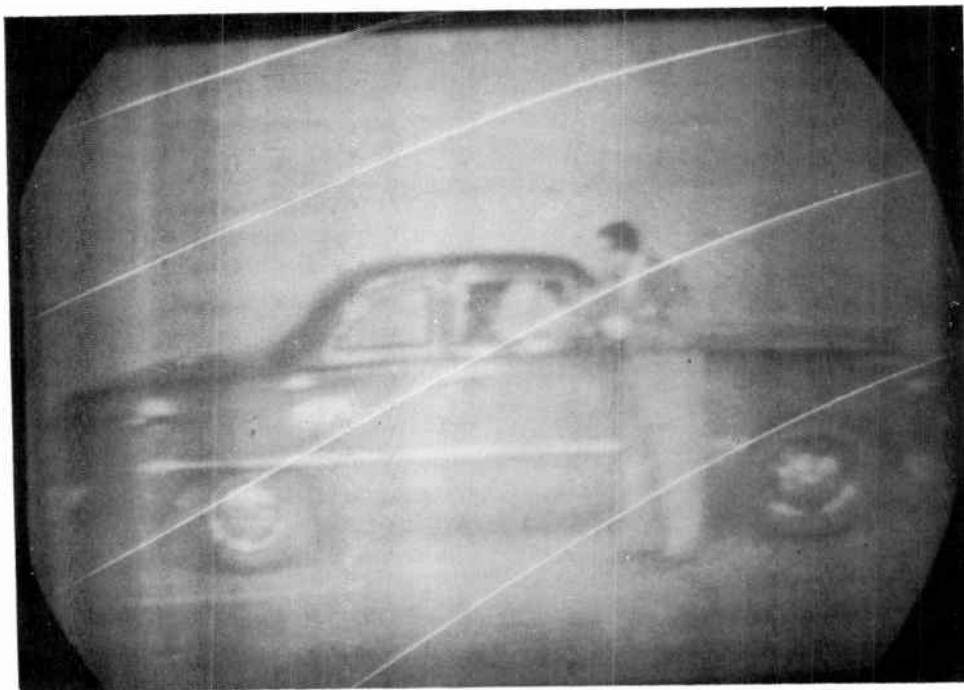
Fig. 94-5. Vertical retrace (slanting) lines on a picture. Note, incidentally, that the lines are uniformly spaced, indicating good interlace.
