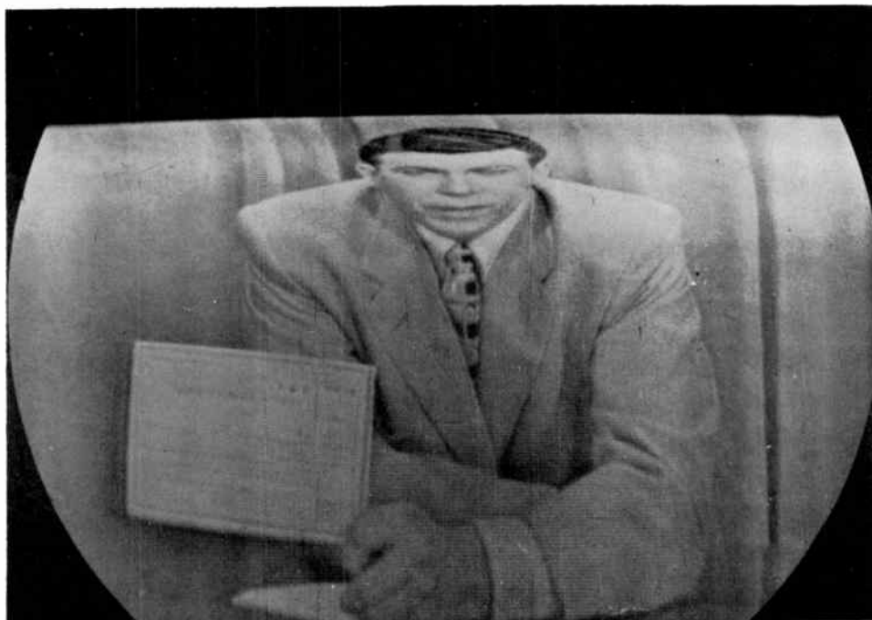
Fig. 93-13. Vertical non-linearity may cause crowding at the top. The more closely spaced trace lines then cause excessive brightness at the top.
