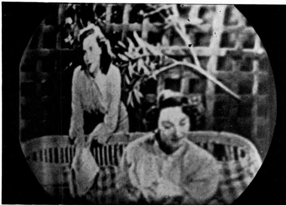
Fig. 93-9. Horizontal non-linearity here causes crowding at the left and stretching at the right.
