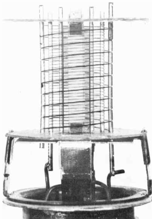
Fig. 11-4. The suppressor is wound around the outside of the screen.
