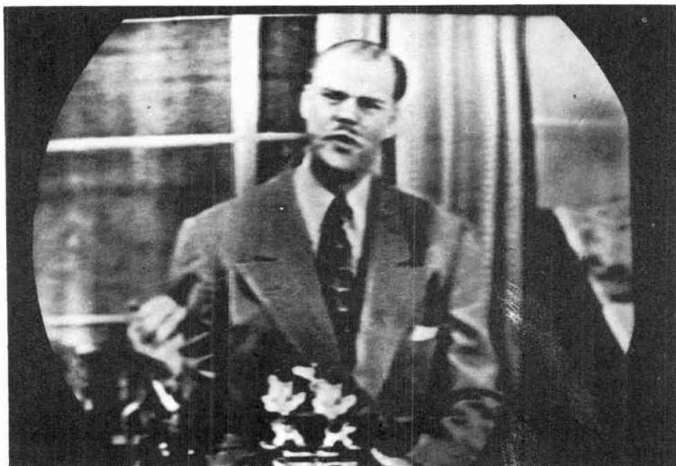
Fig. 93-3. Resolution or definition is poor. This is not due to incorrect focusing, but rather to lack of gain at the high video frequencies and inability to reproduce sharp changes of illumination along horizontal trace lines.
