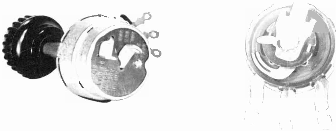
Fig. 25-11. A combination volume control and line switch.
