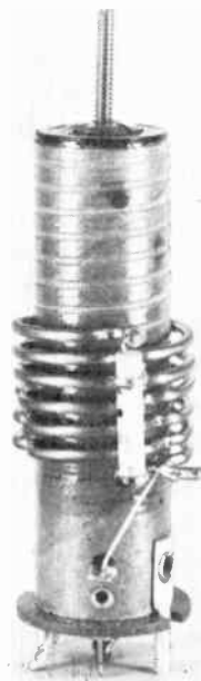
Fig. 80-3. A sound takeoff coupler used with a dual channel sound system.
