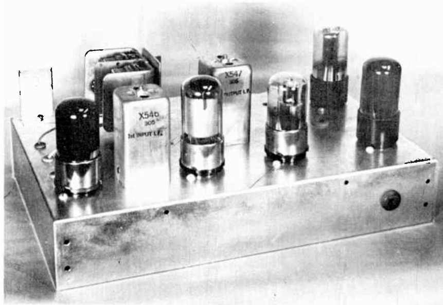
Fig. 77-3. The i-f transformers are enclosed within shielding cans which ground to the chassis.
