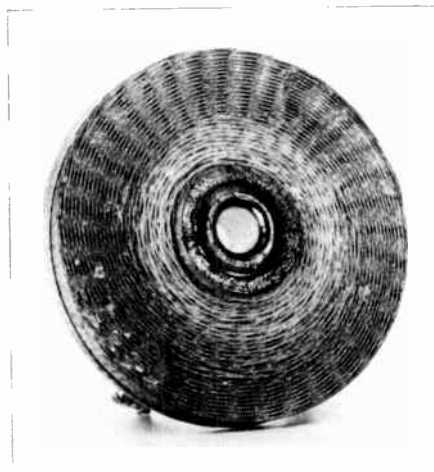
Fig. 17-11. An air-core choke coil used at radio frequencies.
