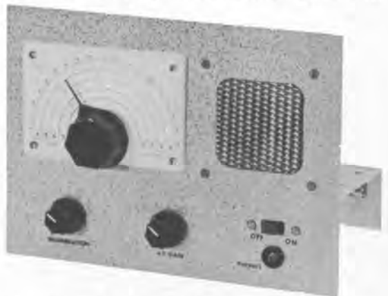
Above: Front view of the complete receiver. Output may be directed to either the internal speaker or a pair of headphones. Frequency range is from 550KC to 20MC.
