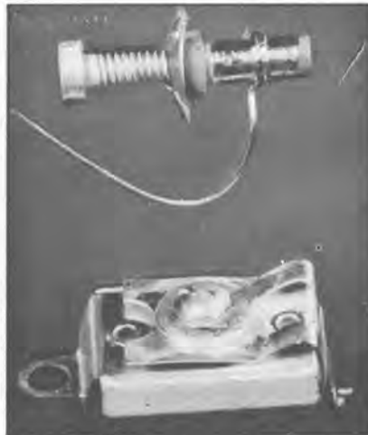
At the top is a ceramic trimmer in which capacitance between the outer metal layer and the screw increases as the latter is turned into the tube. Below it is a typical "trimmer" capacitor, as illustrated in figure 7.
