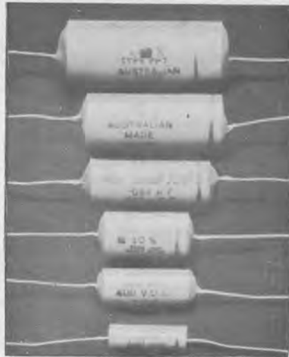
A typical group of modern tubular paper capacitors. These are widely used in electronic equipment though, for critical applications, designers may prefer capacitors having a plastic dielectric.
