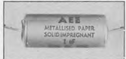
In a "metallised paper" tubular capacitor, the metal foils are replaced by a continuous metallic film deposited directly on the surface of the paper dielectric.
