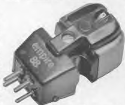
Figure 15: Larger-than-life picture of a magnetic stereo cartridge, with its four output lugs, one pair for each signal channel. The stylus will move both laterally and vertically, though it is not wise to try to verify this by pushing at it with a fingernail. Excessive pressure may well damage the stylus suspension.
