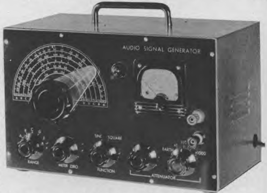
An audio generator which will deliver either sine or square waves of any frequency between 18cps (sub-audio) and 500KC. The output meter and attenuator controls allow the output to be set to any voltage between a fraction of a millivolt and 11 volts.
