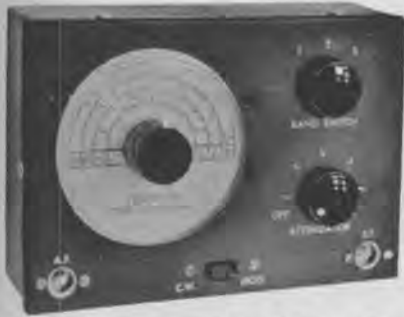
A very compact modulated RF oscillator, intended for the testing and alignment of radio receivers. It is transistorised and operates from a small internal battery.
