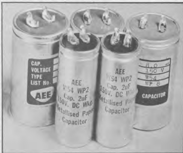
In a "metallised paper" tubular capacitor, the metal foils are replaced by a continuous metallic film deposited directly on the surface of the paper dielectric.
