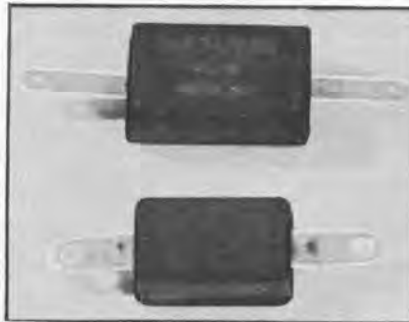
Typical mica capacitors, in which thin metal plates, often of shim brass, are separated by mica sheet, and moulded inside a bakelite casing.
