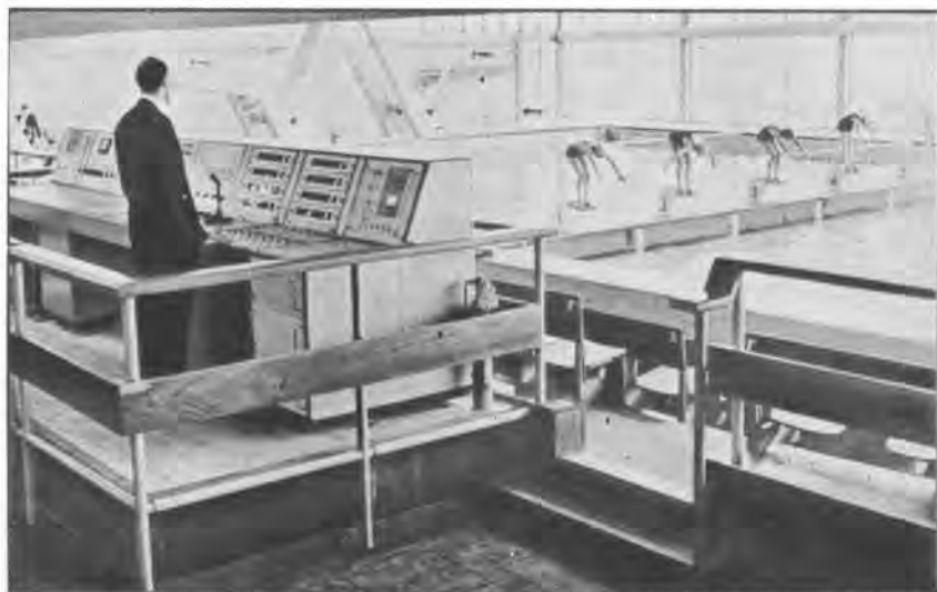
Electronics in sport. At the Crystal Palace Recreation Centre in England, electronic equipment starts and times races to split-second accuracy and stops a swimmer who fails to touch on a turn.
