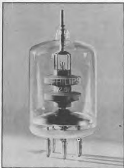
Figure 10. The final RF amplifier stage in a radio transmitter has to handle quite a lot of power, and the valve or transistor used must be arranged accordingly. The valve shown here is a type used in medium-power transmitters, and is air-cooled. In the higher-power transmitters large water-cooled valves are used.
