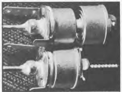
Concentric air trimmer capacitors shown fully out (minimum capacitance) at the top and fully in (maximum capacitance) at the bottom.
