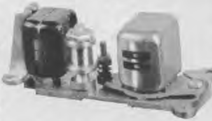
Figure 5: The head assembly from a Collaro tape deck. At left is the erase head and, at right, a head which is used alternatively for recording and replay. Note the separate pole faces for multiple track recording.
