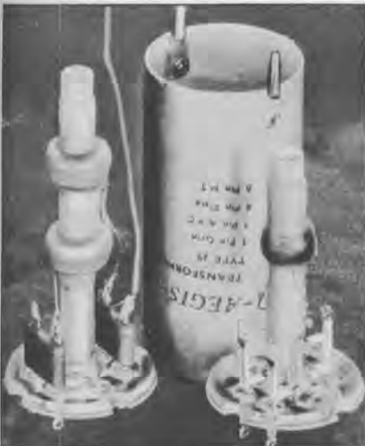
On the left, and withdrawn from the shield can is a typical 455KC IF transformer. The alignment slugs, in this instance, are threaded and screwed directly into the central former. At right is a conventional tuning coil.
