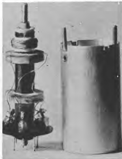
A typical radio type tuning coil, shown withdrawn from and alongside its aluminium shield can. This one has three separate windings, with iron-dust core "slugs" which are adjusted in position by means of the brass screws seen protruding from the top and bottom of the coil former.
