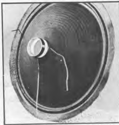
Figure 10: Rear view of a typical loudspeaker cone, with the voice coil cemented to its apex. Special flexible leads connect the voice coil to lugs or terminals mounted on the cone housing.
