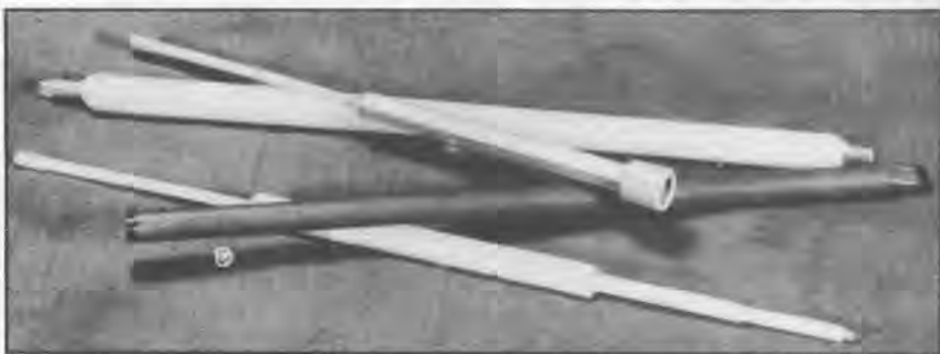
Typical alignment tools used for adjusting radio and television receivers. They are normally non-metallic, or use a minimum of metal, in order to minimise any effect on the circuit being adjusted by proximity of the tool.
