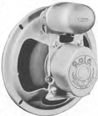
Figure 13: A post-war 6-inch permag. loudspeaker. Magnets can now be made smaller for the same field strength, the latest being the so-called "ceramic" magnets. The loudspeaker illustrated carries its own matching transformer, presenting a load, in this case, of 7000 ohms.
