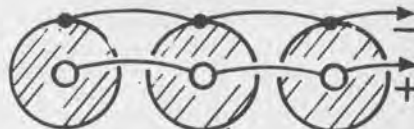
Figure 5. Parallel connection of cells. Voltage remains the same as for one cell but combination has lower internal resistance. It can therefore deliver greater current without serious loss of voltage.
