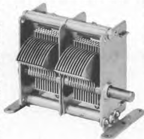
A typical 2-gang variable capacitor. Despite care in the manufacture of such units and the coils that go with them, minor inaccuracies and stray capacitance effects make it necessary to align or "peak" tuned circuits which operate from a common control. Hence this article on alignment.
