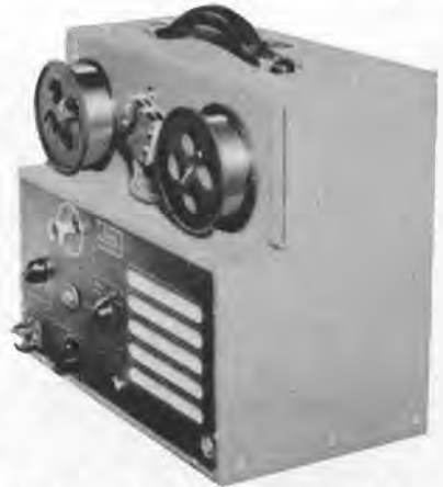
A commercial wire recorder marketed about 1948. Wire recorders were not developed much beyond this stage.
