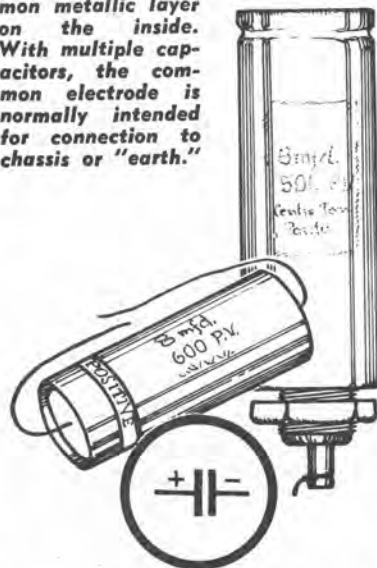
Figure 5: Sketched at right is one of the old can-type "wet" electrolytic capacitors, in which the centre connection normally goes to the positive side of the circuit. At lower left is a conventional tubular type, with the positive end marked on the outer sleeve. Sometimes a plus sign is used, or the end is coloured red.
