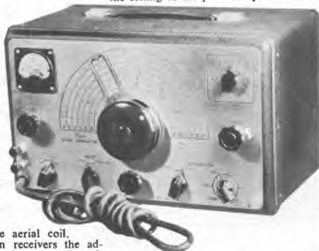
A typical signal generator, providing signals at any frequency between 150KC and 30MC. Panel controls allow the strength of signal to be varied over a wide range, also the depth of modulation.
