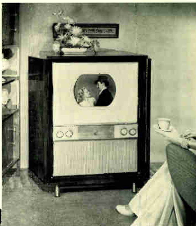
Westinghouse placed color-TV receivers with 12½-inch color kinescopes on the market last February. This is one of the production-line sets.
