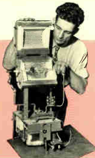
← For movie studios, heaters around mercury lamps when they are not in use ensure readiness for operation without change in light quality.
