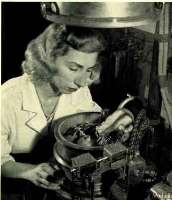
A specimen is placed in the diffraction camera. X-rays scattered from it will pass through the metal foil, and impinge upon film.
