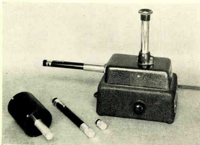
Fig. 3—Ionization chambers (left foreground), and a galvanometer indicator (center) that shows the charge remaining, which is a function of radiation exposure.
