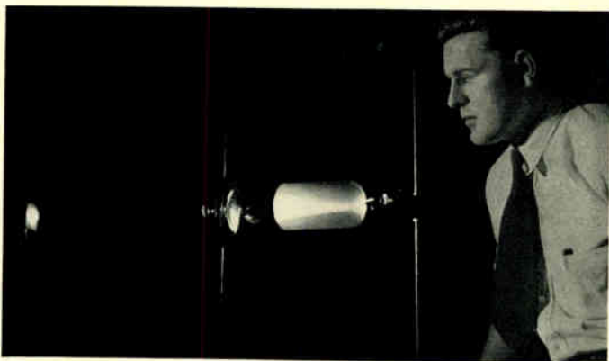
Resonance light from the left is invisible to the camera until it strikes the vapor-filled tube. Atomic absorptions and re-emissions then scatter it in all directions. In picture at right, decay of resonance radiation is measured. Decay curve appears on the screen.
