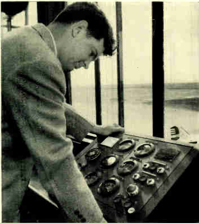
Fig. 4—The ILS instrument panel. ILS brings the pilot to the inner radio marker, at which point he can see the approach lights.
