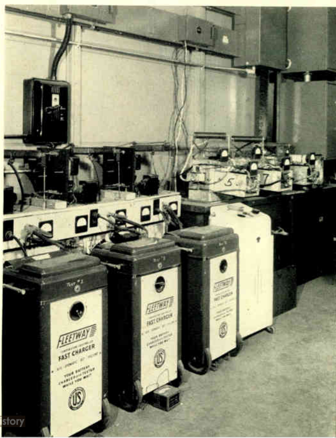
A laboratory arrangement for life-testing selenium rectifiers.
