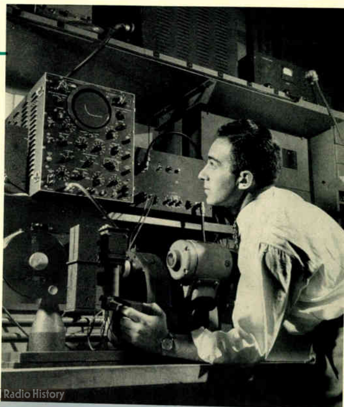
Resonance light from the left is invisible to the camera until it strikes the vapor-filled tube. Atomic absorptions and re-emissions then scatter it in all directions. In picture at right, decay of resonance radiation is measured. Decay curve appears on the screen.
