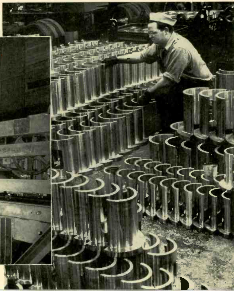
Stretch bending, in which curved members are formed by stressing structural shapes beyond the elastic limit, simplifies manufacture of electric stairways (below). Improved pre-babbitting cleaning makes stronger bearings.
