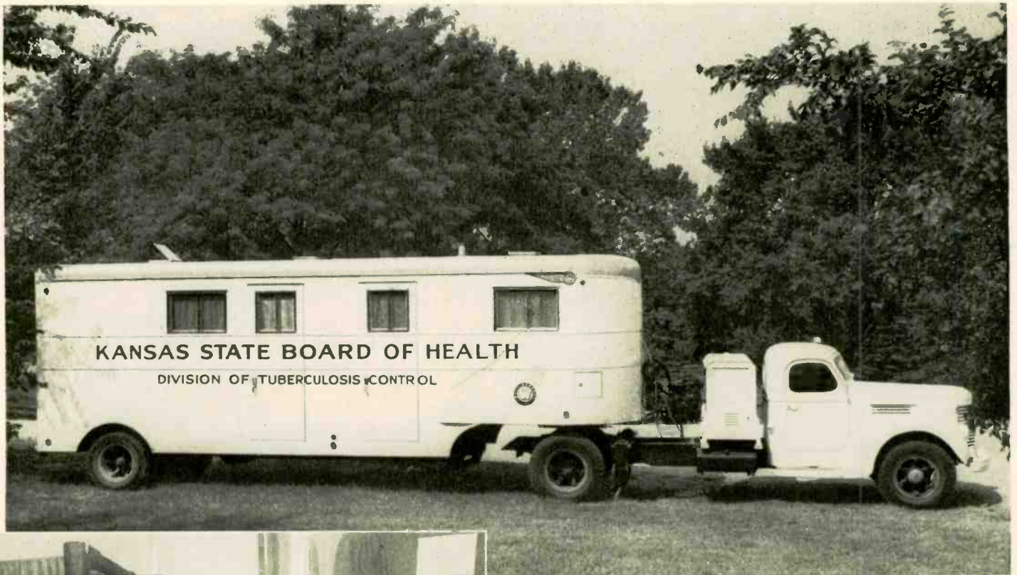
Truck trailers equipped with the photofluorographic x-rays are being used in a nationwide campaign to stamp out tuberculosis. The chest x-ray equipment uses small and inexpensive film, and is equipped for quick handling of large numbers of people. It also contains darkroom facilities.
