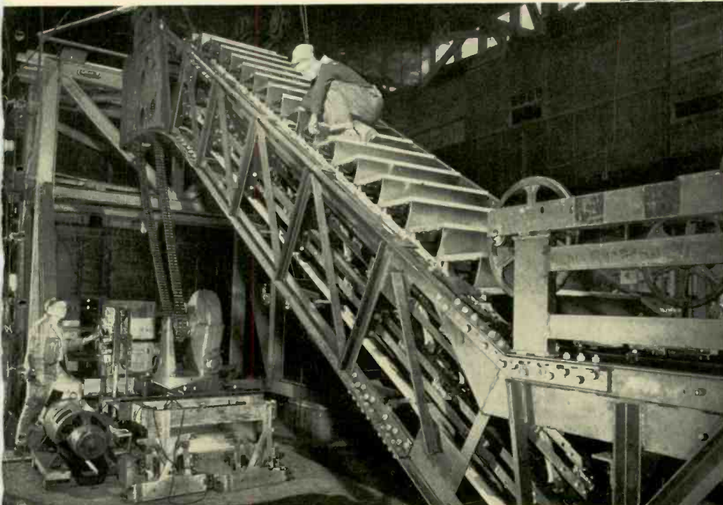
Stretch bending, in which curved members are formed by stressing structural shapes beyond the elastic limit, simplifies manufacture of electric stairways (below). Improved pre-babbitting cleaning makes stronger bearings.
