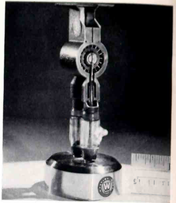
A 3-cm magnetron cutaway to show internal arrangement. The terminals running up from below are for the cathode heater. Power from the wedge-shaped cavities feeds through the vertical slit into the waveguide at the top. A glass window in the flange forms the vacuum seal. To obtain the desired mode of oscillation, alternate cavities are connected by pairs of circular rings.
