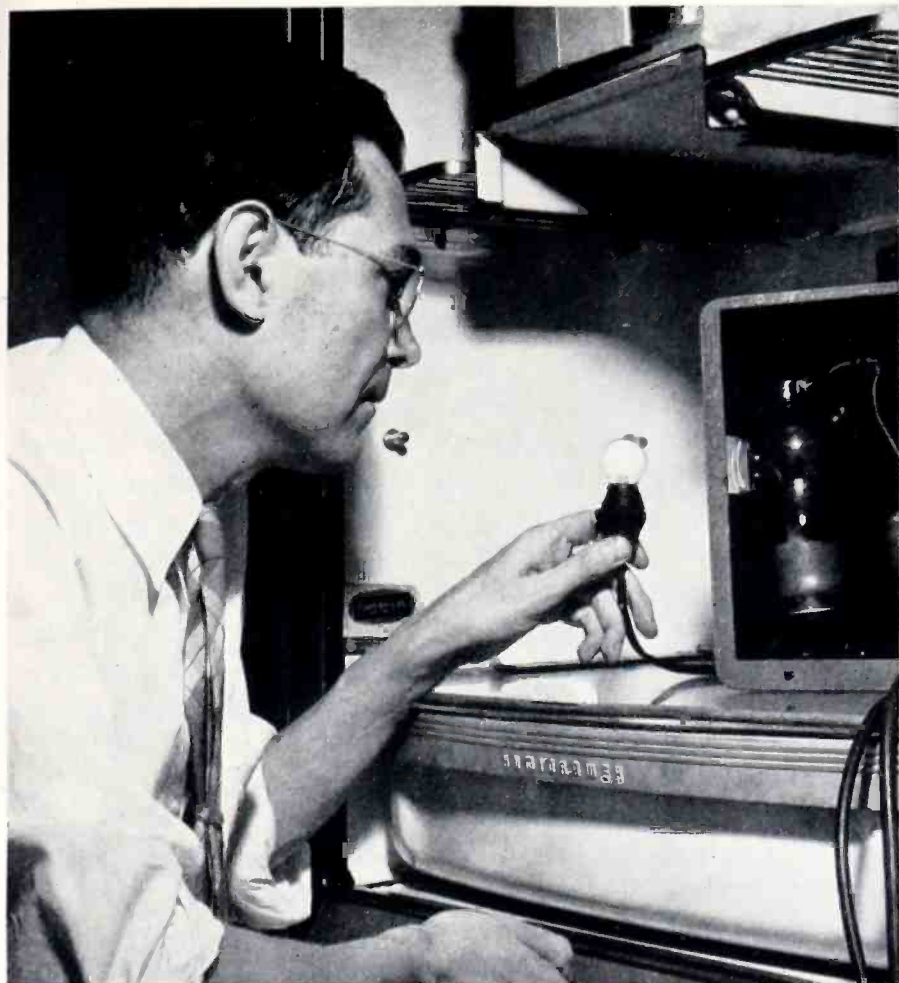
In the Westinghouse Laboratories a research engineer (above) measures the effectiveness of one of the new walnut-size Sterilamps made especially for use in refrigerators . . . (upper right). A pocket-size publication, the Electronics Digest, reduces to simple form the best information relating to industrial electronics . . . (right). As an aid to intelligent planning new or revised hospital facilities, scale-models of x-ray machines and associated apparatus are invaluable.
