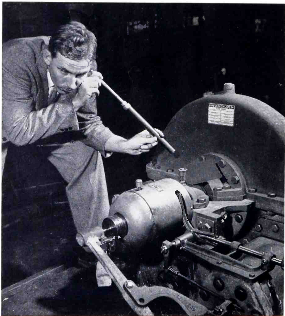
The principle of the doctor's stethoscope has been adapted to a device for checking performance of high-speed machines. It is a resonance tube devised particularly for steam turbines. By changing the effective length of the telescopic resonance sections, sounds indicative of any malperformance are made clear.
