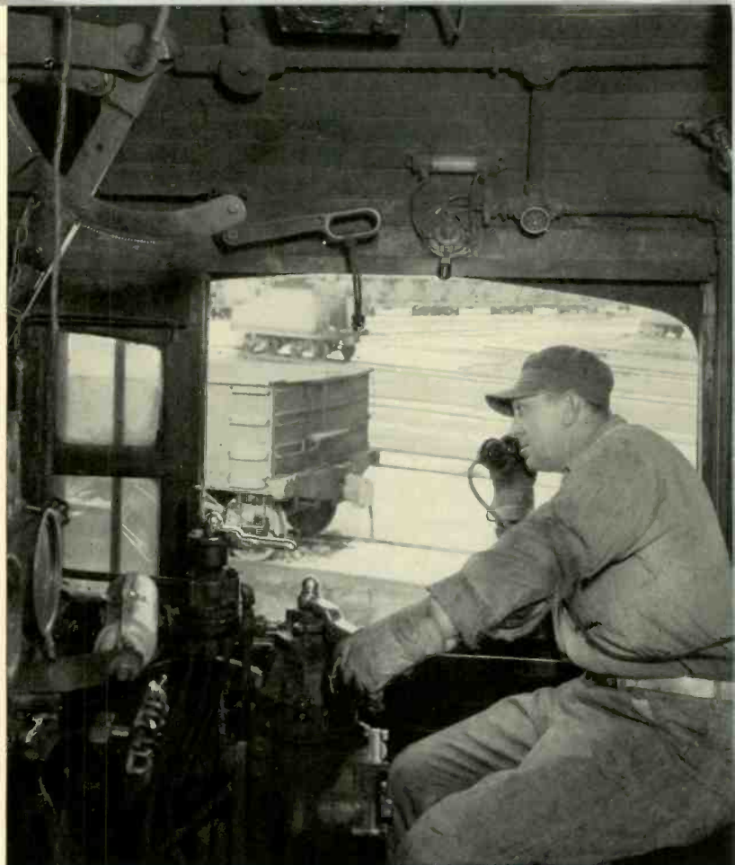
Voice communication between crews at front and rear of trains and to wayside signalling towers, long a dream, has become a practical reality.
