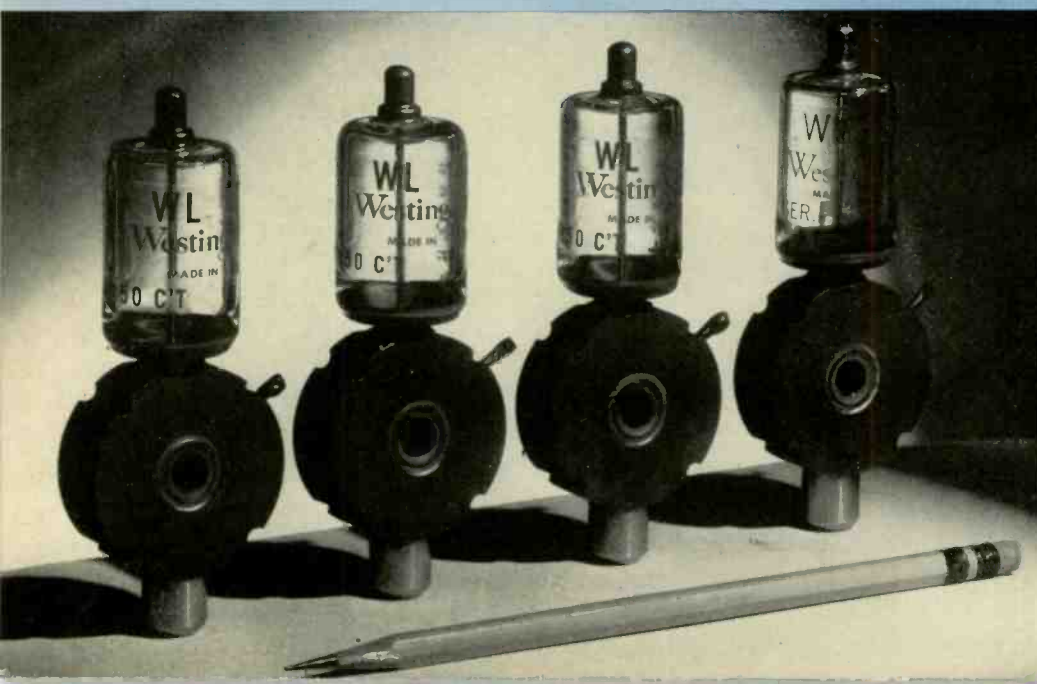
Below are super-speed devices that switch radar receivers to and from the antennas a thousand times per second. At right is a 2-kw oscillator (partial cut away) for high-frequency heating.
