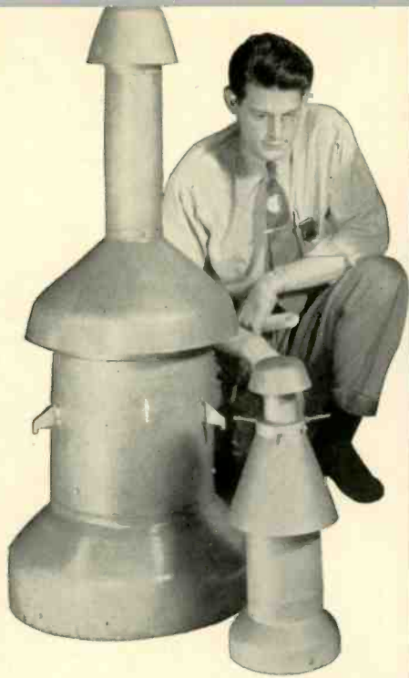
Extremely low vacuums are obtained by diffusion-type pumps. Above are the internal cones of two sizes of diffusion pumps.
