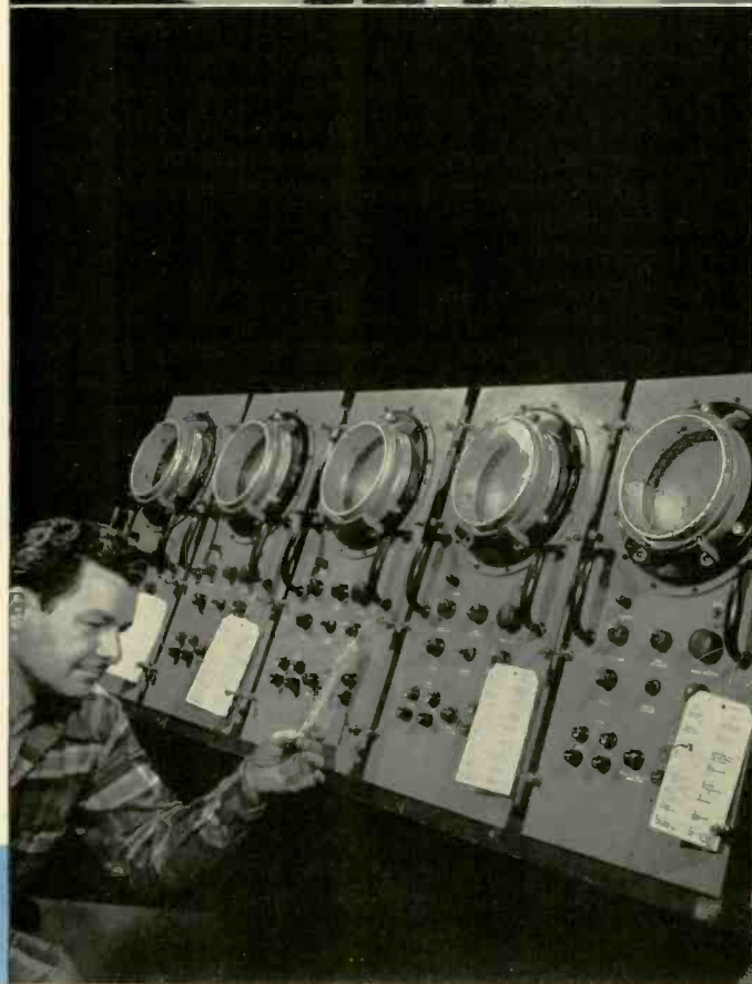
Radar antennas take many forms, even like the skeleton of a large umbrella. At right, a few of the thousands of radar receivers, with plan-position-indicator scopes, march down the assembly aisle.
