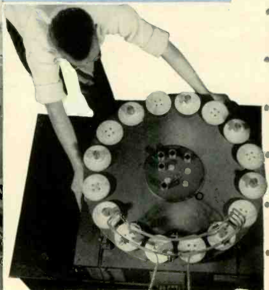
The electronic high-frequency laboratory is a busy place. Below, short metal cylinders on a rotating table are being inductively surface hardened.
