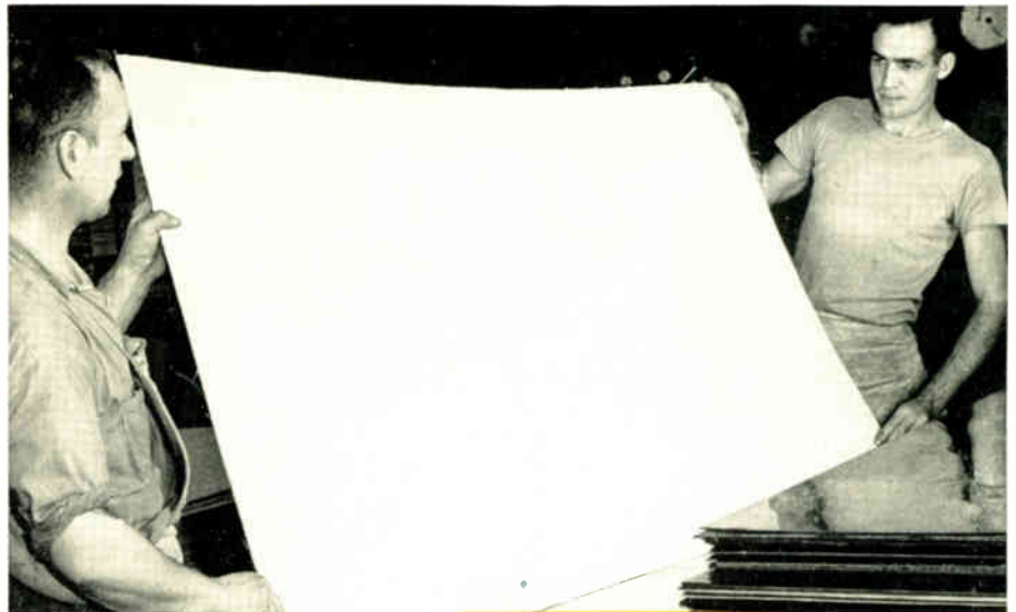
The melamine impregnated glass cloth panelboards emerge in dazzling white sheets from the ponderous forming presses.
