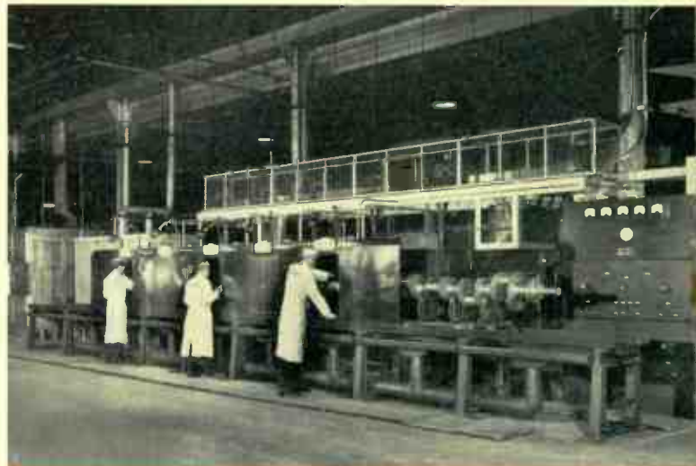
Fig. 9—Extra long shafts are hardened in a tunnel line, a long machine with an inductor block for each bearing, all controlled from one panel.
