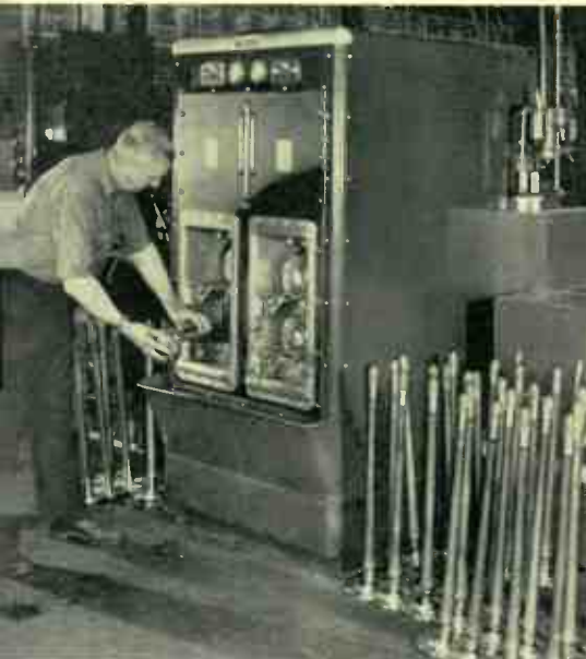
Fig. 10—Certain surfaces of an automobile axle shaft are hardened and made into bearing races. Two shafts are here hardened simultaneously.
