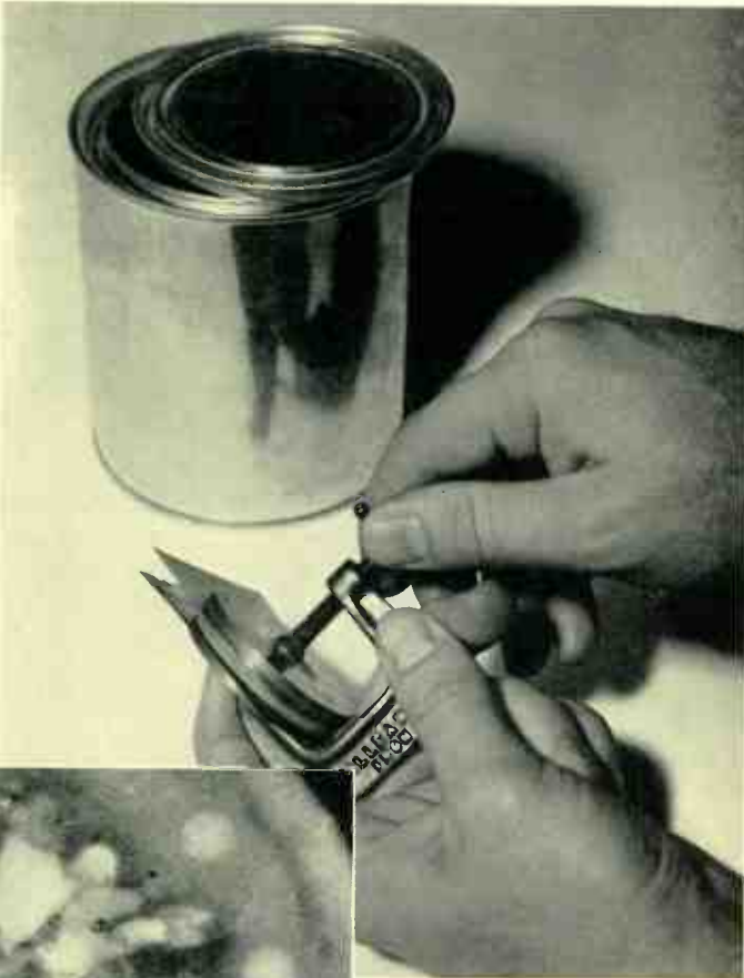
The light areas on the microphotograph (left) show the concentration of phosphorus around blowholes in steel, as photographed with the exceedingly simple "tin-can-and-clamp camera" (above).
