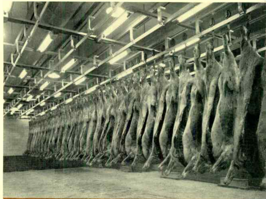
The long lamps produce bactericidal radiation that reduces mold formation. Meat is kept in prime condition longer; trim loss is less.
