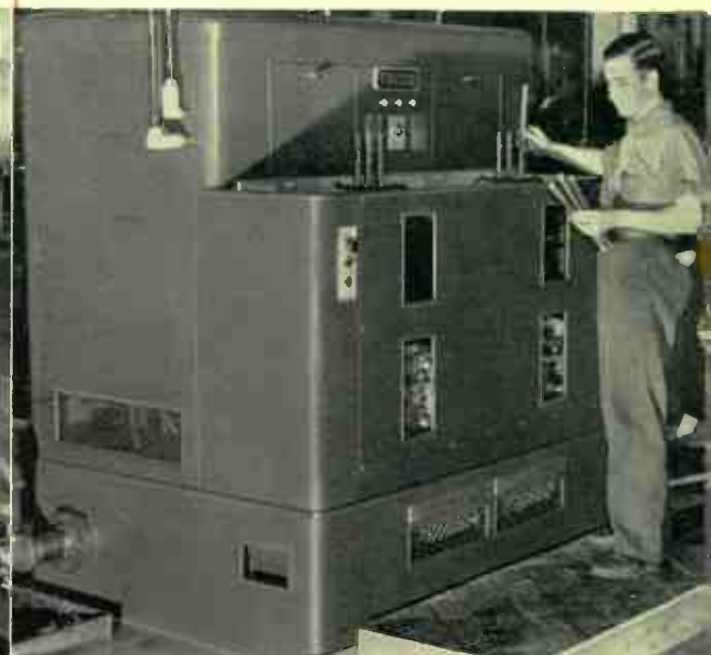
Fig. 12—Three automobile-valve rocker shafts and nine bearing surfaces are heat-treated simultaneously in this fast semi-automatic machine in Michigan.
