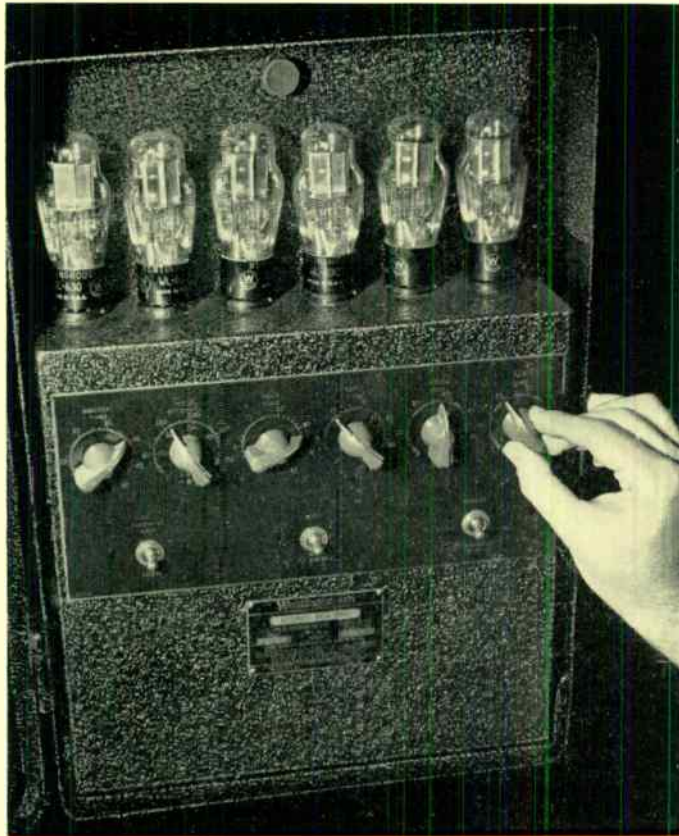
This precision electronic timer automatically divides the time required for a spot weld (1/2 to 2 seconds) into the several shorter periods necessary for the component operations.
