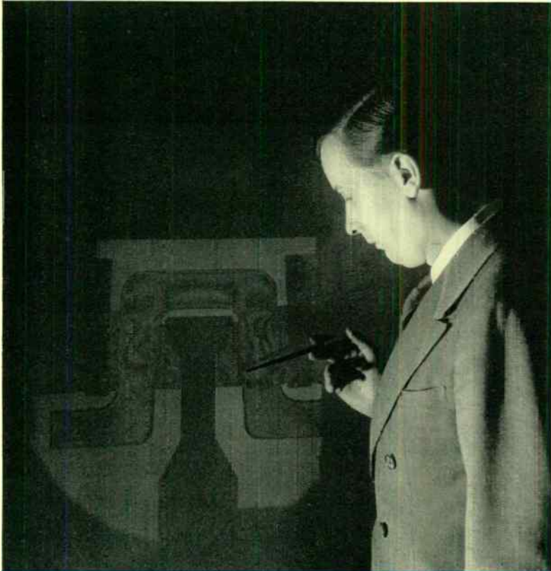
Photoelasticity of porcelain insulators is being studied for the first time by Dr. M. Hetenyi. Here the projection of fringes caused by polarized light shows the distribution of the mechanical stresses that occur in a large bakelite model of a porcelain insulator mounted on its pin.
