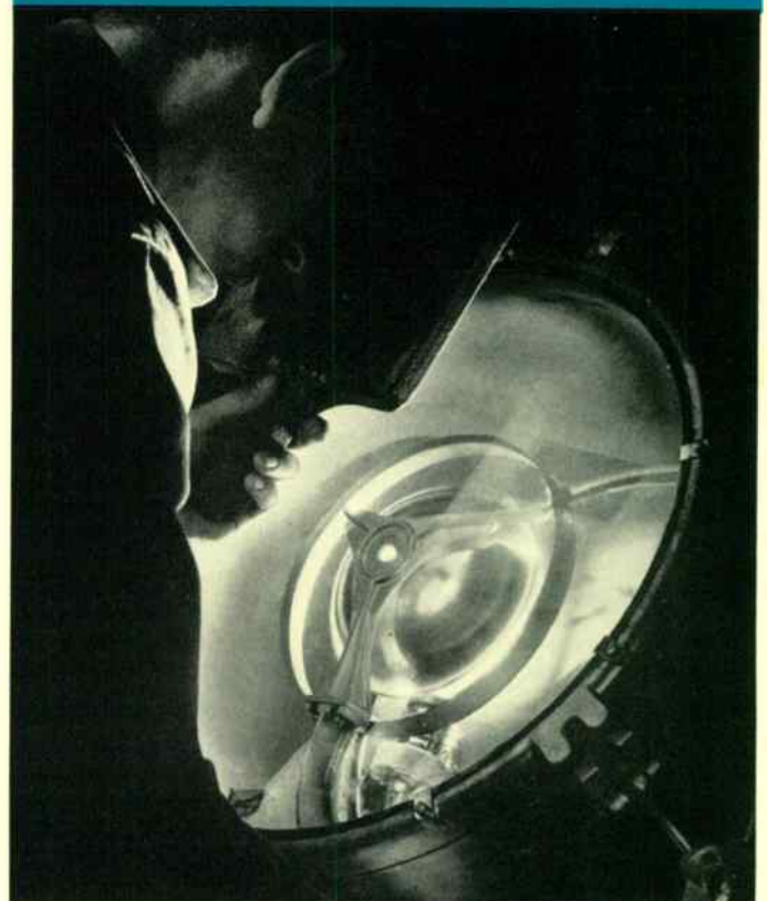
Adjusting the filaments in a new 16-inch searchlight designed primarily for marine work and other long-range spotlighting.
