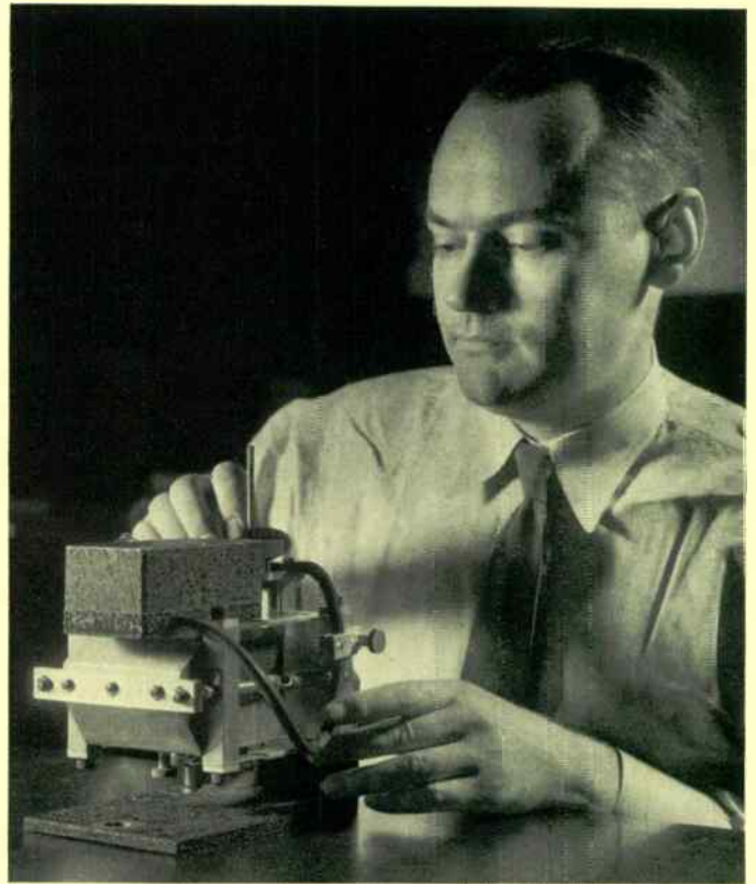
Vibration pick-up for balancing low-speed rotors.
