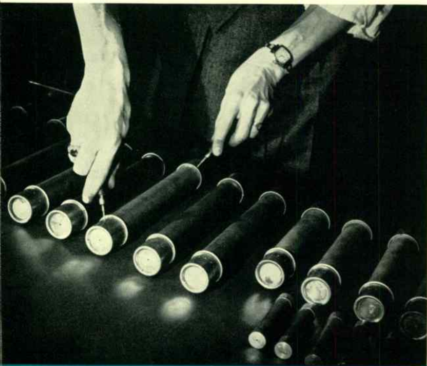
A new type boric-acid fuse eliminates the need for external current-limiting resistors, providing compact protection for potential transformers, especially in metal-clad switchgear.
