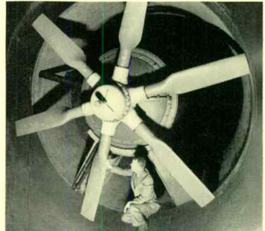
The 13-foot propeller of the Wright Brothers wind tunnel at Massachusetts Institute of Technology is driven by a 2000-hp induction motor.
