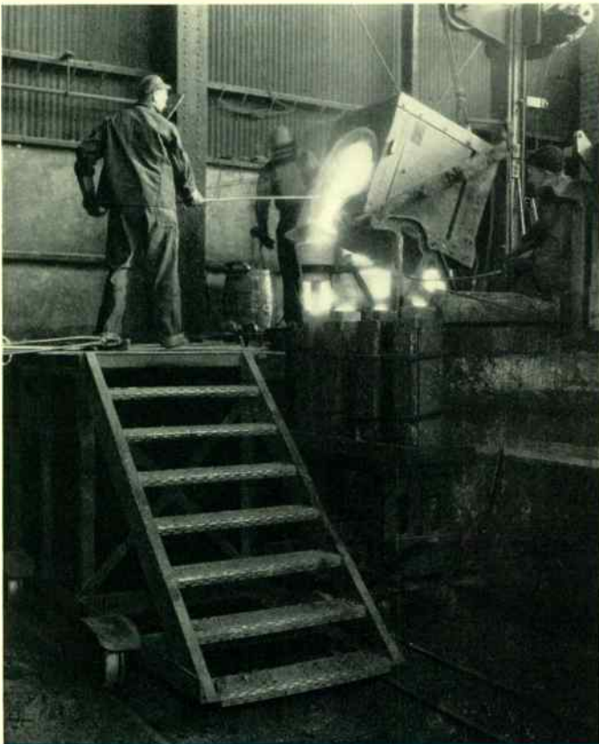
The Carpenter Steel Co. of Reading, Pa., employs induction heating to make high-speed tool steel and to remelt stainless steel.
