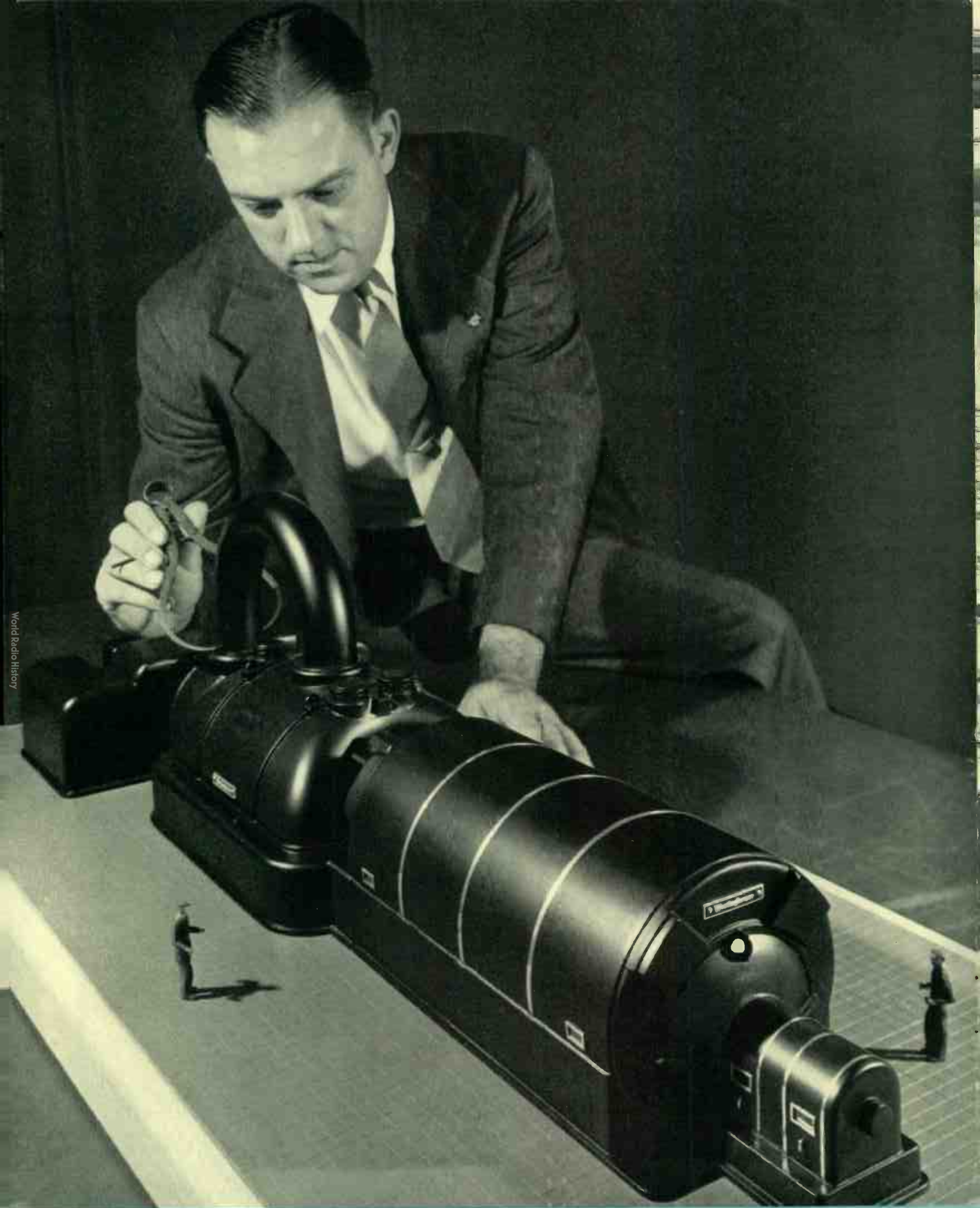
From "toys" engineers learn how to make machines look better. Here industrial designer D. L. Hadley is with a model of a large hydrogen-cooled turbine generator.
