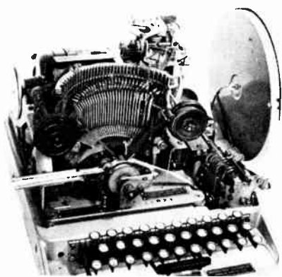
Typing mechanism with ink ribbon on Western Union tape teleprinter
