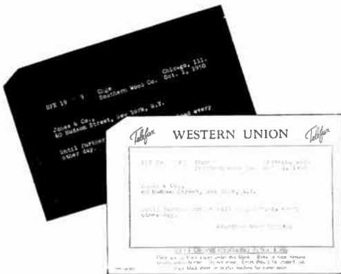
Sending blanks used with "stylus" Desk-Fax transceiver. White wax solid ink is transferred to black conductive paper from back of white blank
