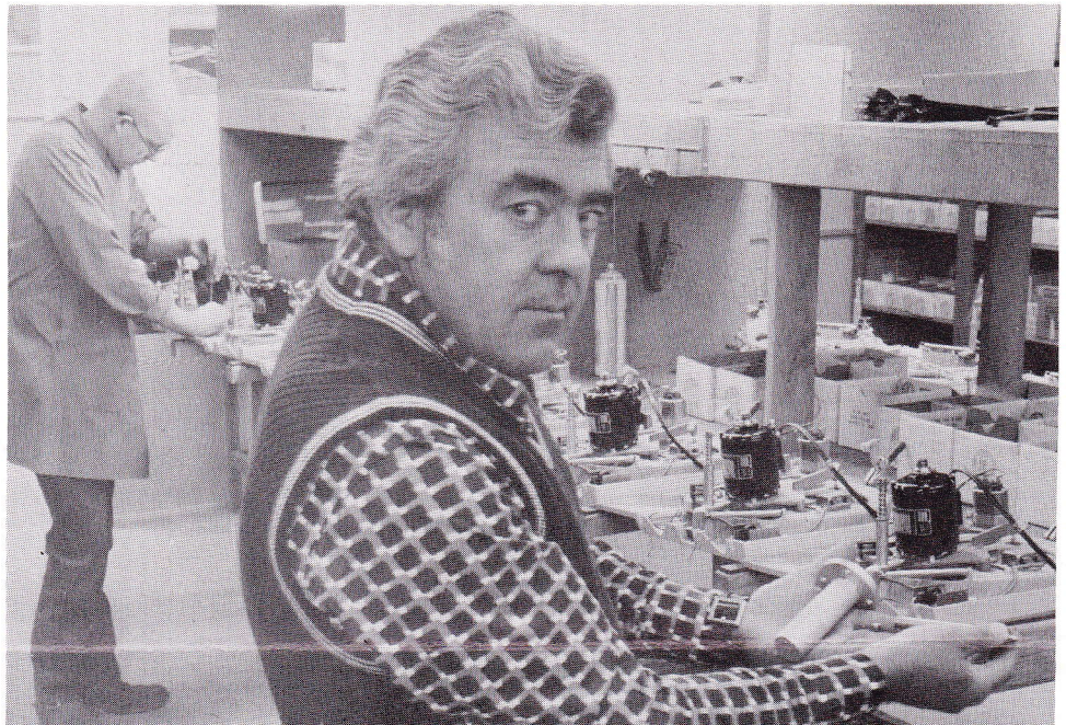
JOHN FERNANDEZ , Sparta mechanical engineer, shows the unique heart of the GT12 Turntable. The shaft is pressed into the platter and the assembly seated in the well on the ball (left hand) with .005'' tolerance or better when assembly completed. Machining tolerances of platter rim, shaft, and well run as close as +.0000'' to -.0001'' to achieve complete interchangeability of stock parts. Ray Dickey, (in background) pretends to ignore his boss to continue assembly work. —Sparta Photo
