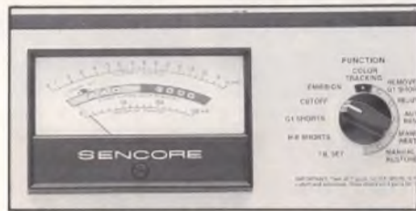
Fig. 10: The CRT must adjust into the cutoff box if it is going to produce an acceptable picture. A tube that won't reach cutoff has a cathode that is heavily worn in the center.
