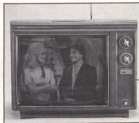
Fig. 7: Would you watch this picture? Even with the brightness and contrast controls at maximum, this picture is still dark and dull. Restoration is the only hope for this television.
