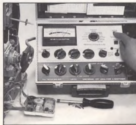
Fig. 11: To restore a tube with weak emission, begin with Auto Restore. Hold the Restore button down until the CR70 completes 3 cycles of restoration.
