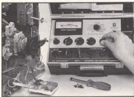
Fig. 9: Before restoring a CRT, test it first so you know which restoration level to use.
