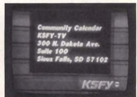
Fig. 2: A cathode worn only in the center causes the deep blacks and silvery whites that most technicians call a "gassy" tube.
