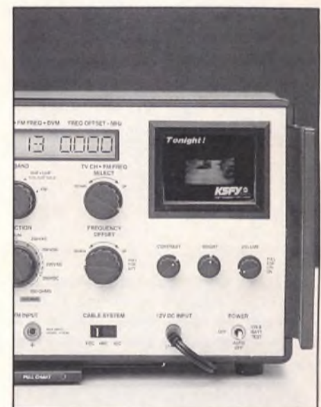
Fig. 6: The wideband monitor on the FS74 CHANNELIZER SR. lets you find the source of the noise problem, since you can see exactly how it affects the picture.
