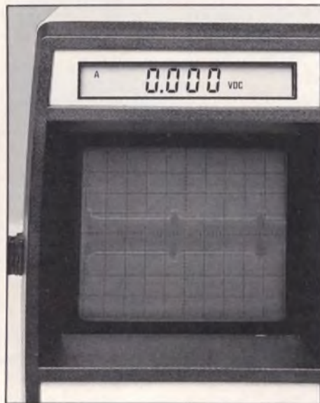
Fig. 5: Most conventional FS meters measure the video carrier incorrectly, because the carrier is only at full amplitude during the sync pulses. Horizontal sync is present only 7.5% of the time.
