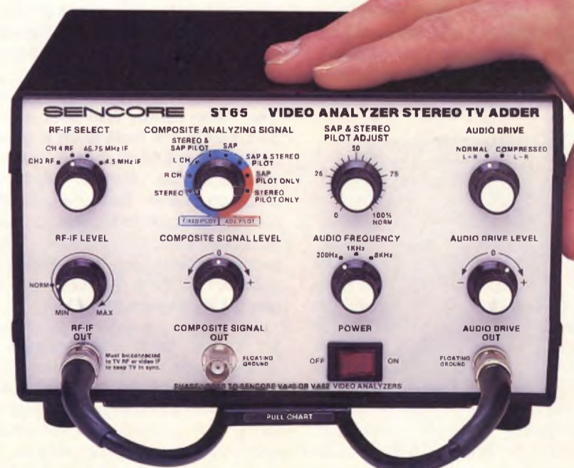
Fig. 2: The New ST65 Video Analyzer Stereo TV Adder can update your VA48 or VA62 Video Analyzer for stereo TV and VCR service. It has the special substitute signals, outputs, and modulation needed for successful stereo service.
