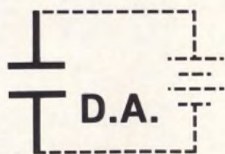
Fig. 5: Dielectric absorption prevents a capacitor from fully discharging because it acts like a small battery is inside.
