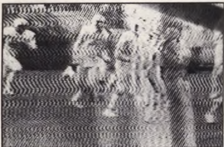
Fig. 3: These are three examples of problems that show up in the FS74 monitor, which are tough to find with a meter or spectrum analyzer: a) Ringing in the picture, b) Ghosts, c) Co-channel interference.
