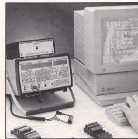
Fig. 16: The AUTO-Z's built-in computer is easily adapted to the IEEE488 interface bus. Use your personal computer to add automatic Z Meter applications to your test system.
