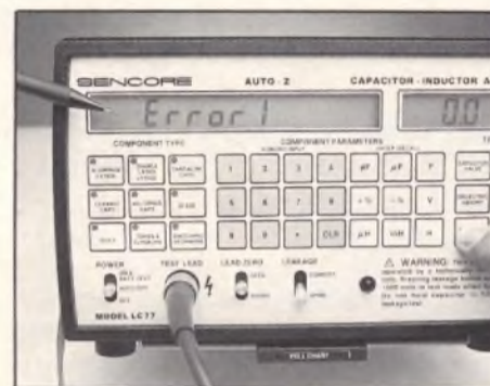
Fig. 9: If you try to perform a test incorrectly, an error message shows on the LCD display to alert you to the exact problem. Each error message is explained in the AUTO-Z's handy pull chart.
