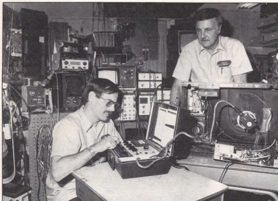
Fig. 1: Mal Hodgdon watches as Stan, his "Master Tech" restores a CRT. "I've given orders here that every TV that comes in here is to have the tube tested first thing . . ."
