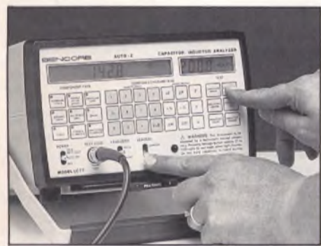
Fig. 13: High voltage resistors are above the range of ohmmeters; the AUTO-Z measures leakage to 1,000 Volts, with the readout you need. Simply select CURRENT or OHMS to analyze leakage or resistance to 1,000 Megohms.
