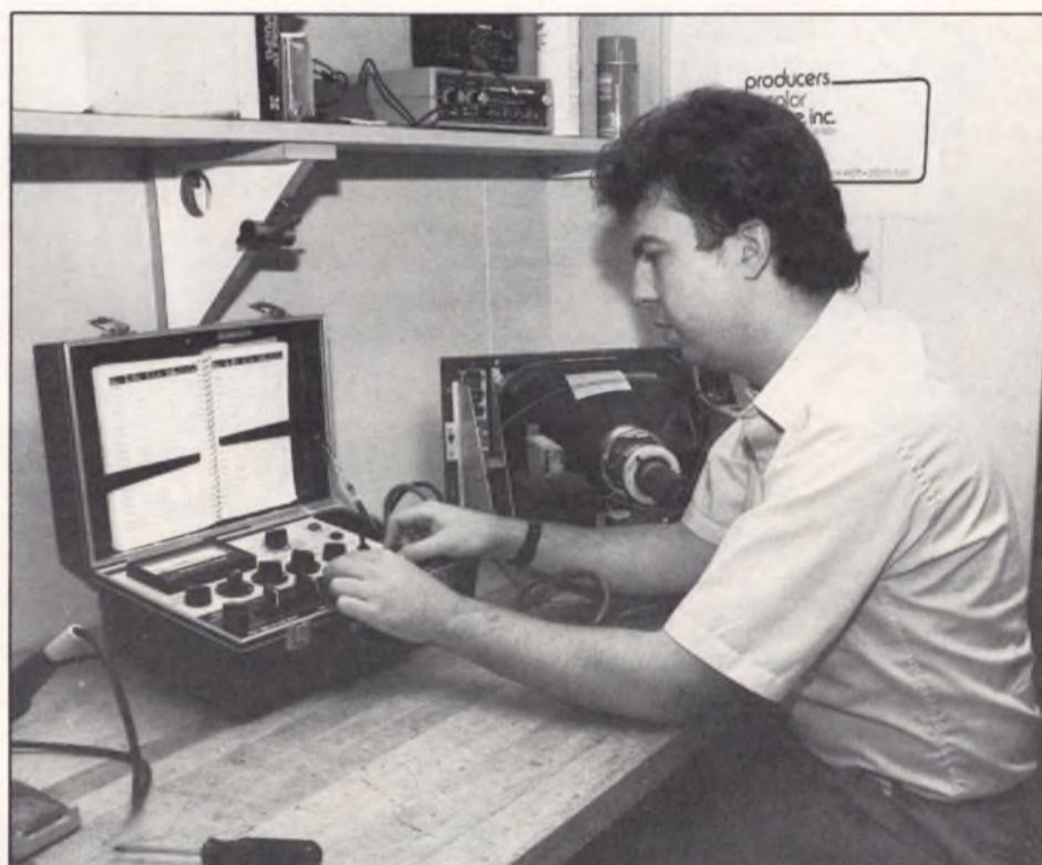
Jeff King of Producers Color successfully restores video monitor tubes which cost about $1,000 a piece to replace. "Usually the total life of a restored tube is three or four years, so roughly that's a savings of $250 for each tube."
