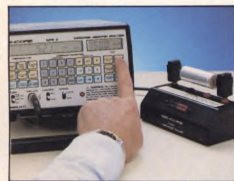
Fig. 3: After testing thousands of capacitors, Sencore Engineers have proven that capacitors show leakage problems more reliably when tested at their full rated voltage.
