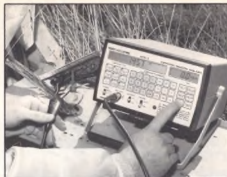
Fig. 14: Battery operation lets you analyze capacitors, coils, resistors, and transmission lines in the field or on a mountain top - 1,000 VDC test output makes the Z Meter the only portable dynamic LCR tester on the market.
