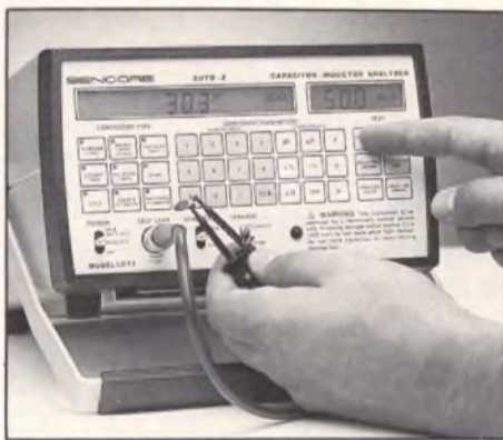
Fig. 10: The AUTO-Z includes test ranges that cover every capacitor or coil you'll want to test, now or in the future. No other tester measures caps from 1.0 pF to 20F and coils from 1 uH to 20 H.
