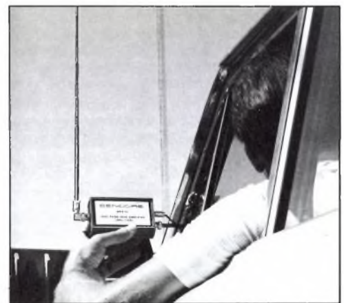
AN210 Adjustable Antenna. . . . $25.00 Supplied with FC51 but not FC45. Used to pick up very small signals. Plugs into 50 or 1 Megohm input jacks.
