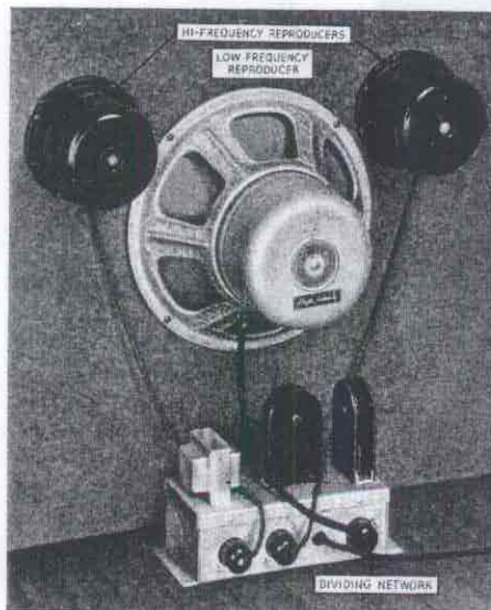
Special Four Unit Speaker System Available for Scott Phantom and Philharmonic Models.
