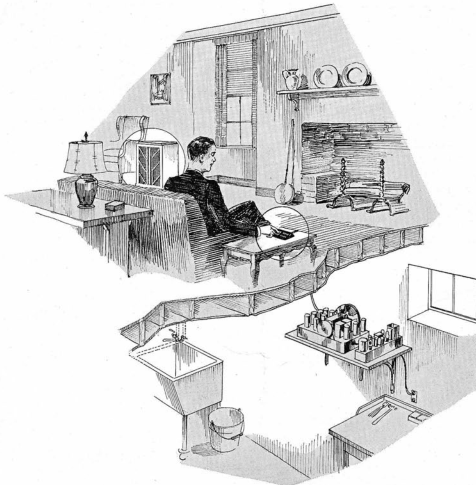
View Showing How Scott Telematic May Be Installed in Basement, and Operated in Living Room.
