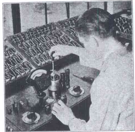
THE OSCILLATOR AND ANTENNA COILS ARE MATCHED PERFECTLY ON THE PRECISE APPARATUS SHOWN, WHICH CAN MATCH COILS TO WITHIN \frac{1}{8} OF A TURN IN A COIL OF 90 TURNS.
