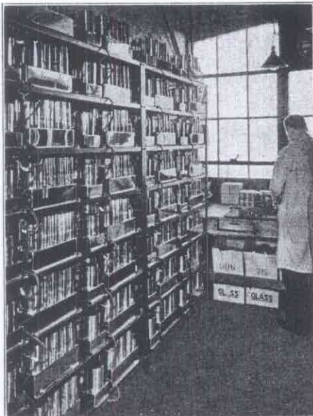
AFTER THE INITIAL TEST AND CALIBRATION, EACH SCOTT RECEIVER IS PLACED IN THESE "AGEING" RACKS AND GIVEN A 24 HOUR CONTINUOUS OPERATION TEST, TO MAKE CERTAIN THAT EVERY PART IN THE CIRCUIT IS PERFECT.
