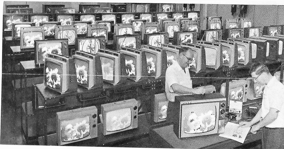
Figure 1—TV Life Test Area at Electronic Tube Division Plant at Emporium, Pennsylvania.
