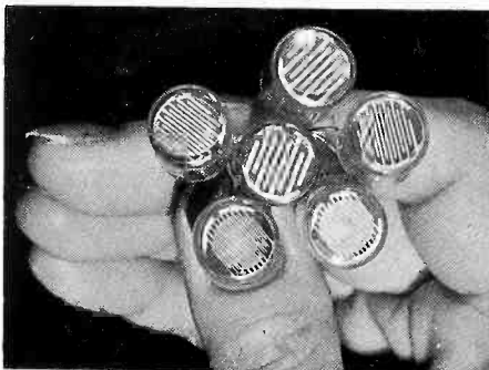
Figure 1—Sylvania T-4 photoconductor. Hermetically sealed all glass envelope protects sensitive wafer against moisture.
