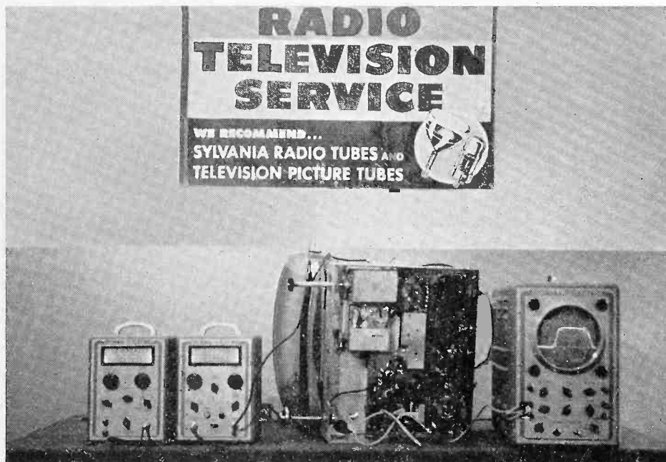
Figure 1. TV alignment set up. From left to right is the Sylvania 500 sweep generator, 501 marker generator, Sylvania TV set and Sylvania 400 oscilloscope.
