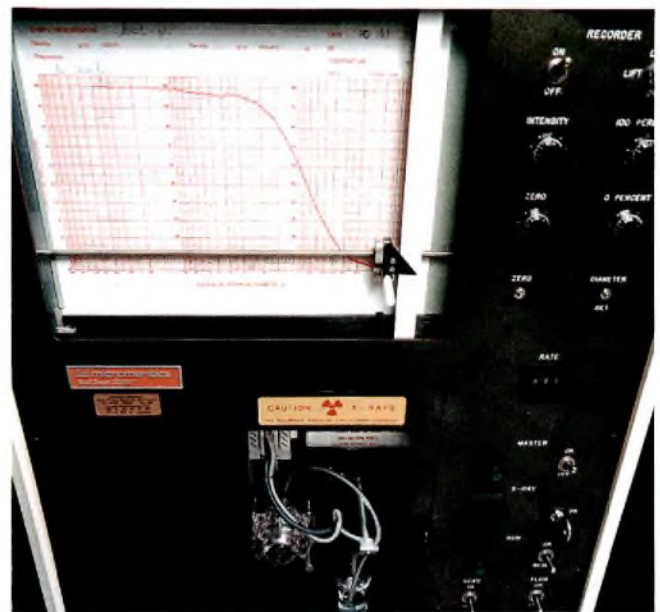
Fig.3 The equipment shown here meters particle size to ensure that we use only the highest grade ceramic
